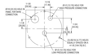
4. MOUNTING: The Photohelic® Switch/Gage may be either panel mounted or surface mounted.
