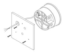
B. SURFACE MOUNTING: Drill (3) 3/16" dia. holes for mounting screws and (1) 7/8" dia. hole for wire assembly as shown in hole location drawing. Insert screws from rear of panel and thread into tapped holes on back of Photohelic® case. If rear pressure connections are to be used, make 1/2" dia. holes located as shown in hole location drawing in left column.
