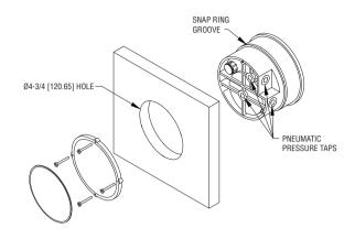
A. PANEL MOUNTING: Cut a 4-3/4" or 120mm dia. hole in panel and insert the complete unit from the front. Slip on the mounting ring and install the split snap ring in the groove on the bezel. Seat the mounting ring against the snap ring and thread the four screws through the tapped holes. Tighten screws against rear of panel.
