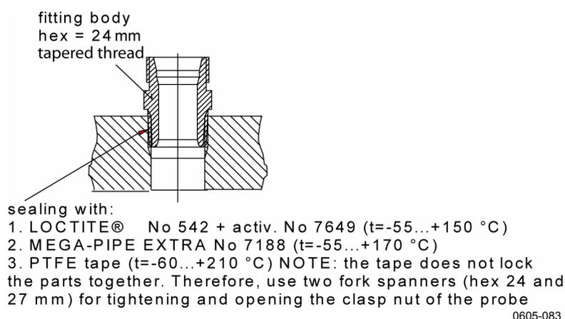
**Figure 6 Sealing Thread Cutting for the Fitting Body**
