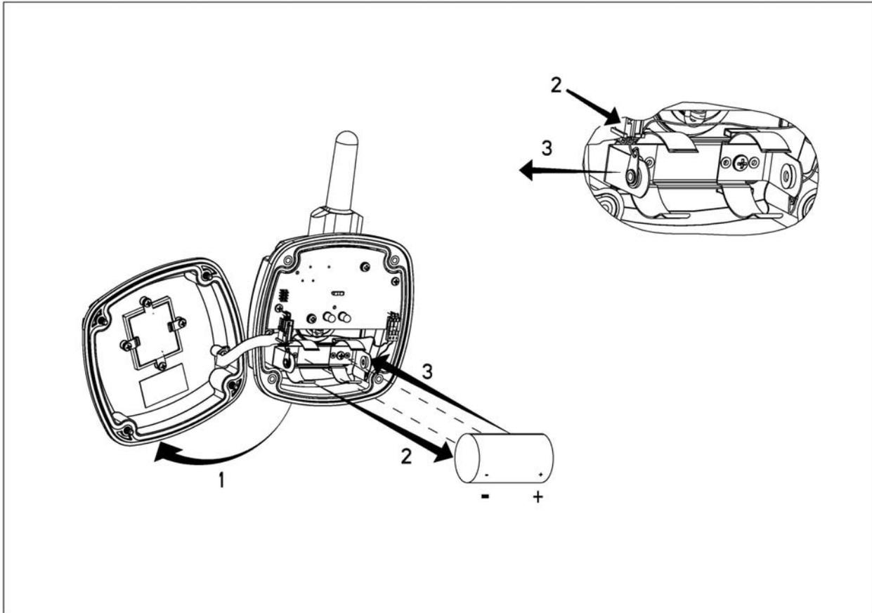
Figure 5-1 Battery replacement
