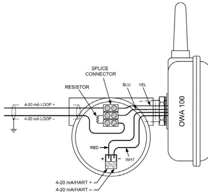
Figure 3-6 OWA 100 – TWO-WIRE CONFIGURATION WITH RESISTOR
