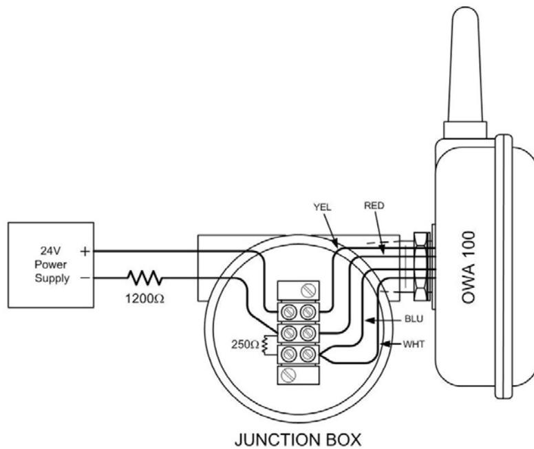
**Figure 3-11 OWA 100 – AS A ROUTER, NO WIRED DEVICE**
