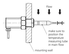
Mounting flange 301 048 For sensors from 160 mm in length
