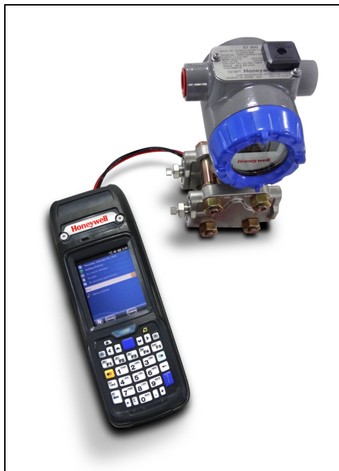
Figure 3-3 Connecting to a device through MCT404
