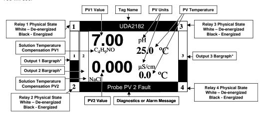
\*On the display, the bargraphs are the outputs in Engineering Units, the corner annunciators are the physical relay states.
