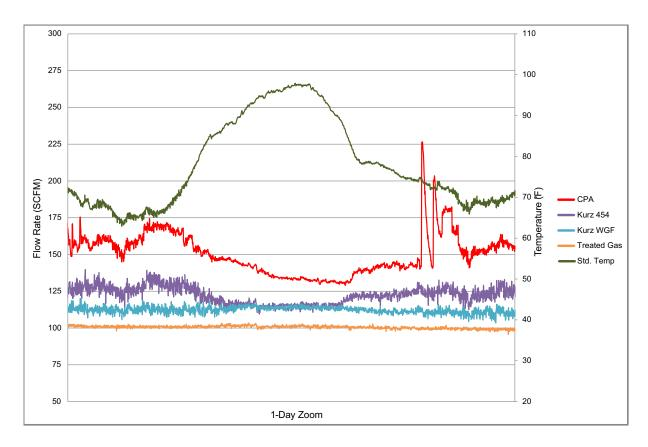
As demonstrated in all graphs, the Kurz WGF outperformed the other thermal flow meters in its realtime monitoring capability of the wet gas flow from the digester. In all positions and at all points throughout the day, the Kurz WGF consistently remained steady with the dry total of the treated gas, and the flow meter maintained a totally accurate reading compared to the dry reading after the cleanup skid.
