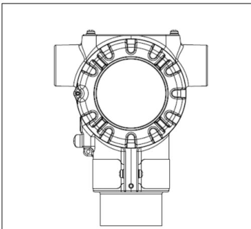
**Figure 3: Electronic Housing Conduit Entries**
