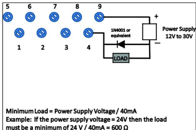
**Figure 9: Digital Output Connections for mA Load**
