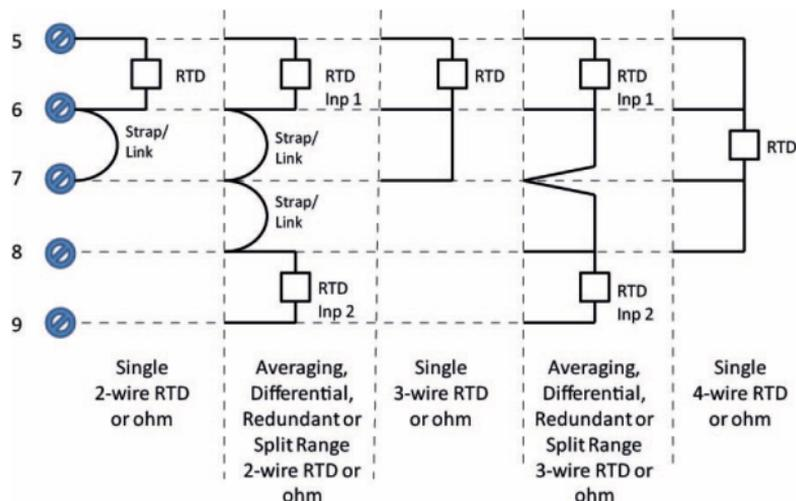
Figure 7: RTD and Ohm Connections
