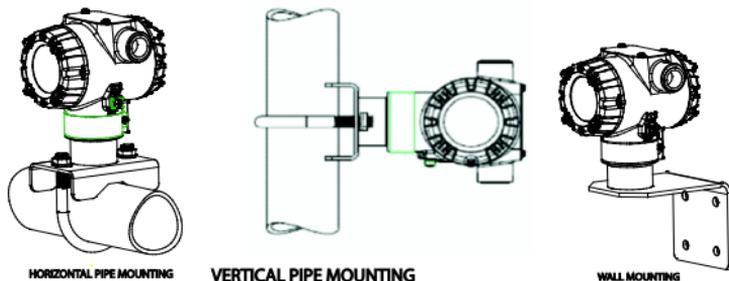
Figure 1: Mounting Brackets
