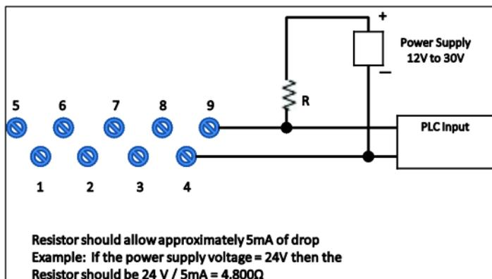
Figure 10: Digital Output Connections for PLC Counting Input
