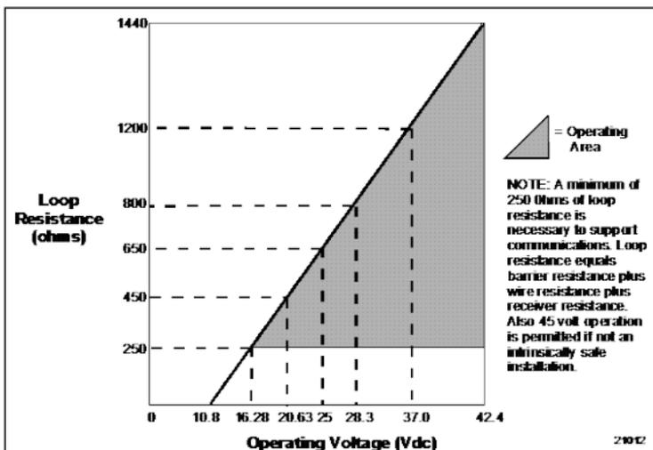
Figure 4: HART Transmitter Operating Ranges
