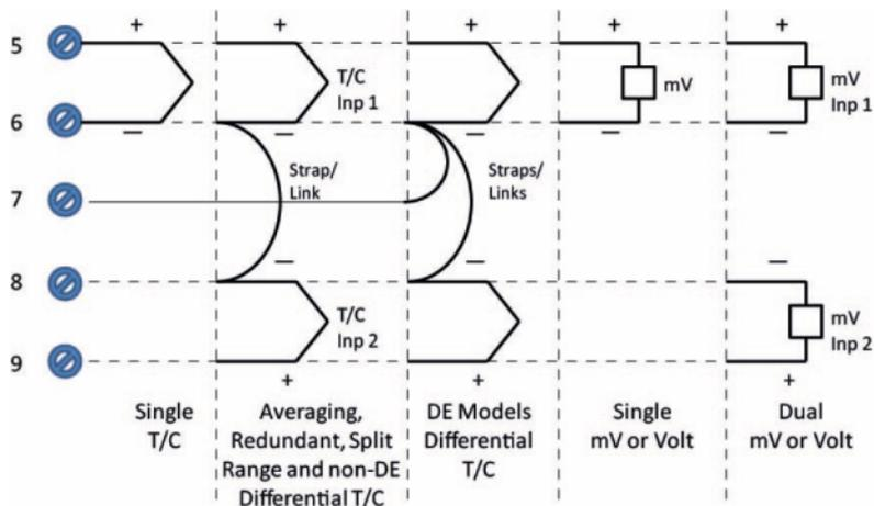
Figure 6: Thermocouple, mV and Volt Connections
