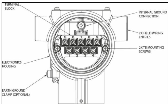
**Figure 5: Transmitter 9-Screw Terminal Board and Grounding Screw**
