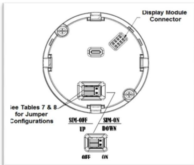
Figure 11: Jumper Location HART/DE
