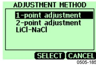
**Figure 18 Example of the MI70 Adjustment Menu**
