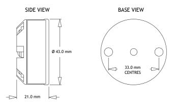
Mounting holes: two holes 5.5 mm diameter, 33 mm centres Centre Hole sensor wire entry: 4 mm
