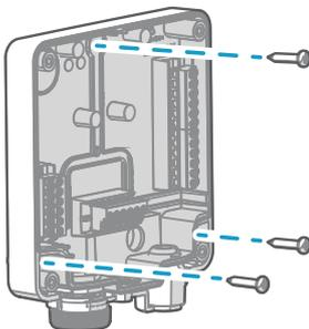
5. Lead the input/output cable inside the transmitter (see [Wiring Options \(page 17\)](#)). If you are wiring through the lead-through on the bottom of the transmitter, test that the strain relief works with your cable.
