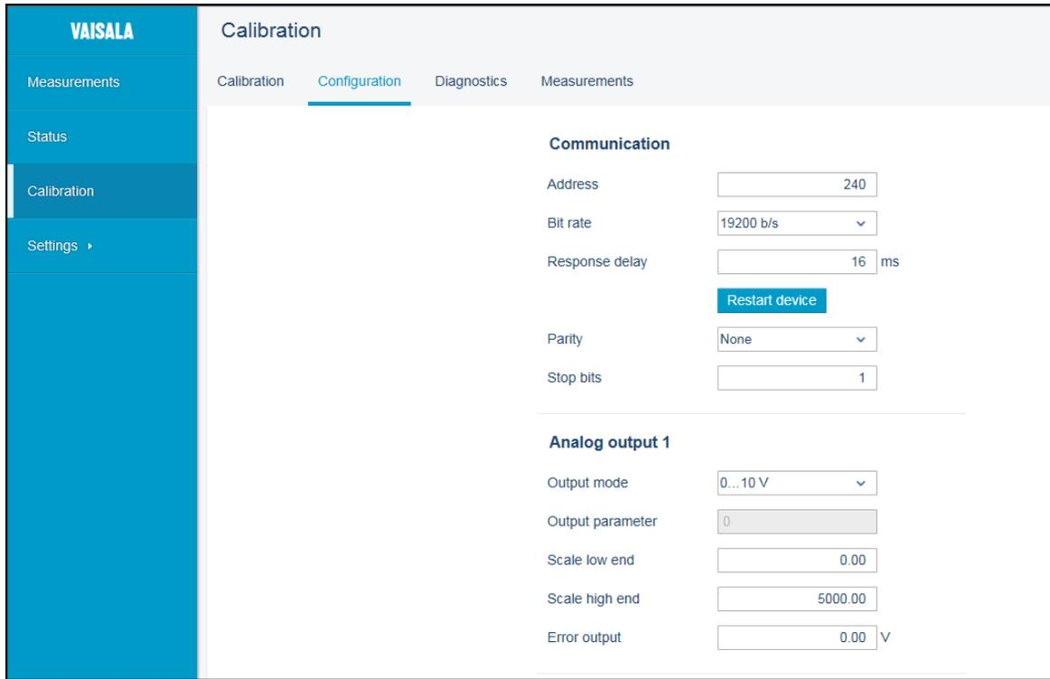
Figure 28 Configuration Tab, CO<sub>2</sub> Probe Example
