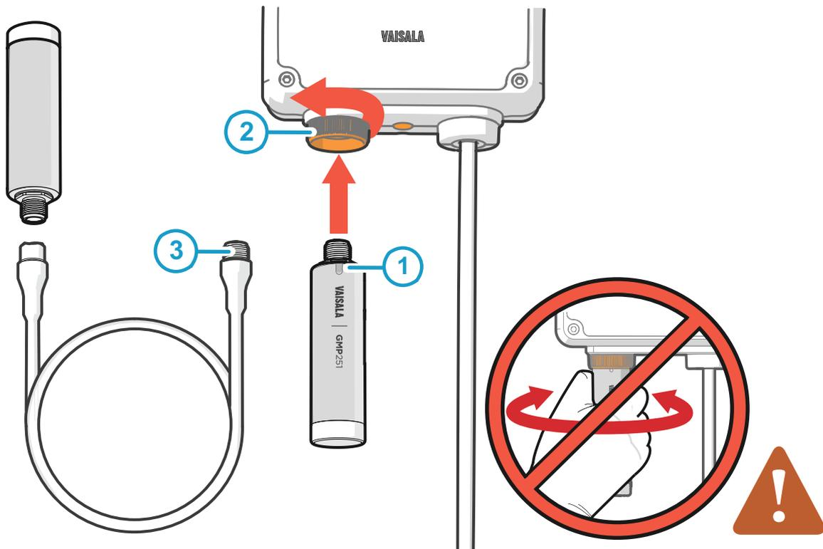
Figure 10 Attaching Probes and Cables to Indigo
