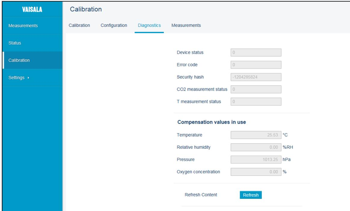
Figure 27 Diagnostics Tab, CO<sub>2</sub> Probe Example
