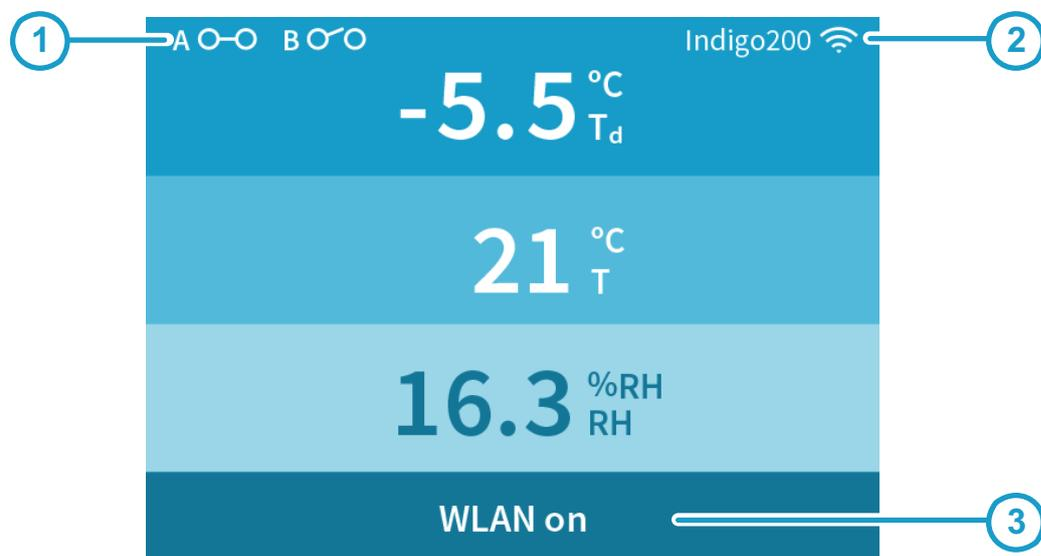
Figure 4 Indigo Display with Relays, Three Parameters and WLAN Notification
