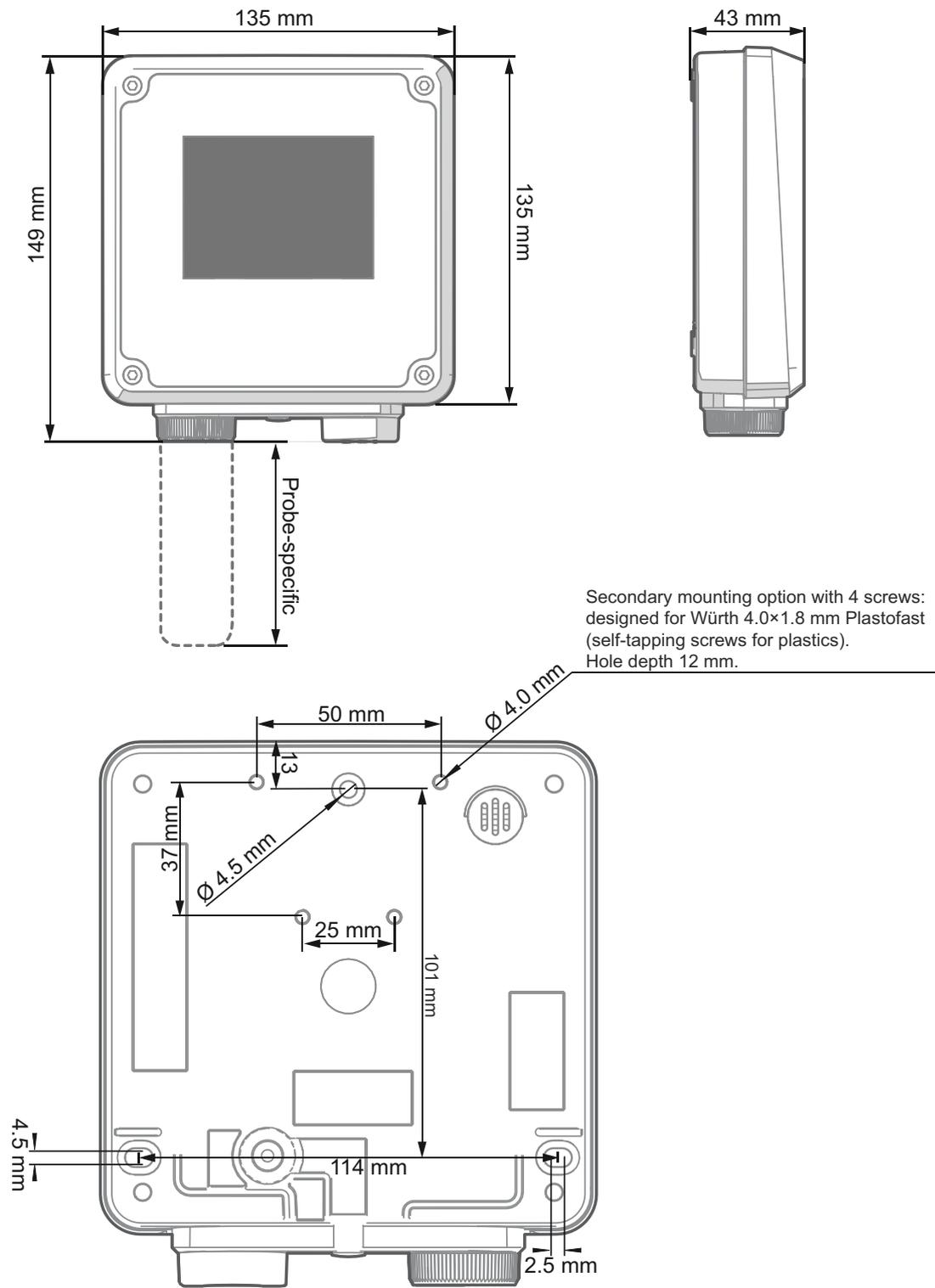
Figure 30 Indigo Transmitter Dimensions in Millimeters (mm)
