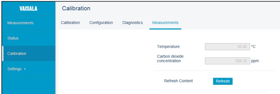
Figure 26 Measurements Tab, CO<sub>2</sub> Probe Example
