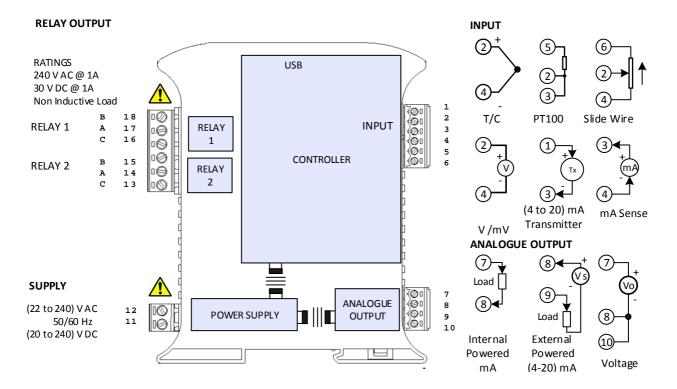
Input connections for cable length >3 metres use screen or twisted pair cables. Thermocouple connections use the correct compensating cable. PT100 connection all wires must be equal length (resistance). Max cable run 30 metres.
