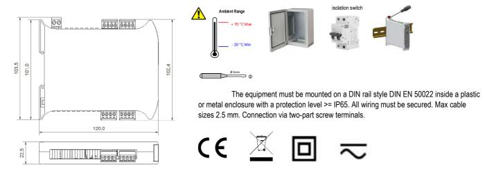
ELECTRICAL CONNECTION - Ensure the supply is isolated before carrying out any installation or wiring. This equipment must be installed by a qualified person. All electrical wiring must be carried out in accordance with the appropriate regulations for the place of installation.
