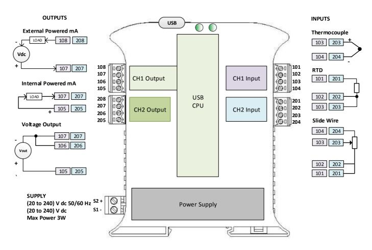
Input Connections For cable length >3 metres use screen or twisted pair cables. Maximum cable run 30 metres.
