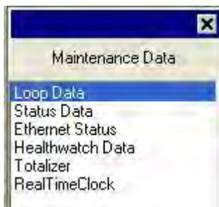
The Loop Data screen allows you to see the current status of each process loop. "OP1, 2 and 3" windows indicate the status of the current outputs. If a current output is not installed, the OP status for that output is always "OK."
