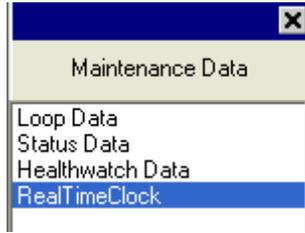
This screen only appears in instruments that have the Real Time Clock option. The Real Time Clock Screen shows both the clock time in the controller and the clock time in your PC. Pressing the “Set Clock” button will set the controller to the same settings as in your PC. It is recommended that units using Email use only this screen to set the Real Time Clock, as that will ensure that the clock and time zone settings used to time-stamp Emails are correct.
