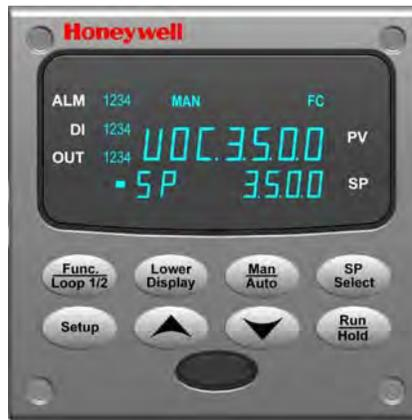
Figure 4-1 Operator Interface
