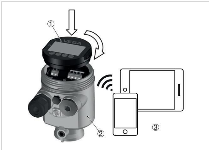
Wireless connection of the sensor to smartphones/tables via Bluetooth
