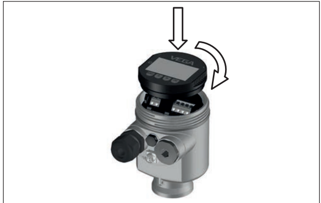
Fig. 34: Installing the display and adjustment module in the electronics compartment of the single chamber housing
