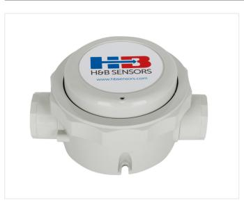
The Type 25 housing is manufactured from plastic and can be used as a junction box or connection head. This plastic housing can be fitted with most types of ceramic terminal block or DIN standard transmitter and is weatherproof to IP67. Additional options include M20 x 1.5, M24 x 1.5, 1/2" BSPP or 1/2" NPT cable entries.
