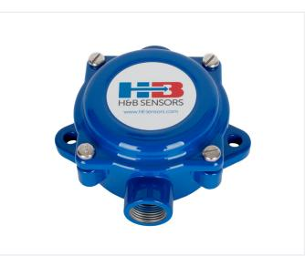
The Type 40 housing is manufactured from high quality aluminium with a tough polyester powder coated finish and can be used as a junction box or connection head. This aluminium housing can be fitted with most types of ceramic terminal block or DIN standard transmitter and is weatherproof to IP65.
