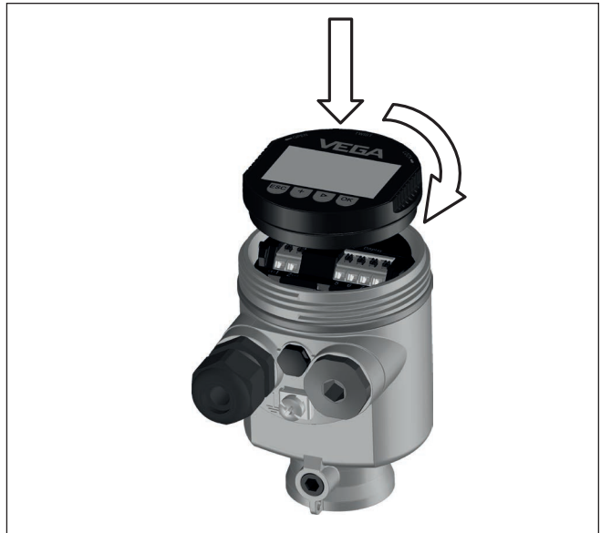
Fig. 6: Installing the display and adjustment module in the electronics compartment of the single chamber housing
