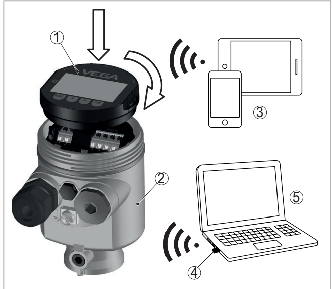
Fig. 2: Wireless connection to standard operating devices
