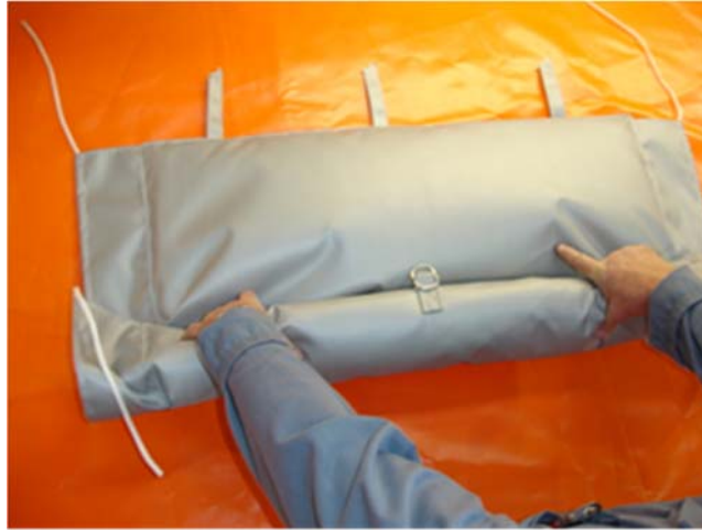
Roll to remove the excess air to assist installation
