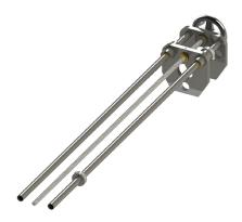
A **restraint** device consists of a u-shaped bracket designed to be used with a Kurz packing gland. The restraint provides a positive lock to preclude pressurerelated instrumentation blowout or an inadvertent blowout caused by a loosened packing nut while the system is pressurized. Process shutdown is typically required should the instrument need to be removed.
