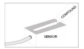
Use the PC4 pipe clamp (supplied) as illustrated above or use a loop of electrical tape for temporary mounting. Apply silicon coupling compound #4 to the coloured face of the sensor. A bead, similar to toothpaste on a toothbrush, is ideal. Do not overtighten (crush the sensor).
