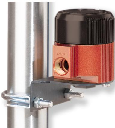
The durable PIH Pressure-to-Current Transmitter provides an economical solution for any process that requires a rugged instrument capable of interfacing a pneumatic device with a data acquisition/control system, controller, recorder, or other electronic instrument. This compact yet powerful unit accepts most pneumatic signals (3-15 psig, 0.2-1 bar, 3-27 psig, etc.) and accurately converts them to a proportional 4-20mA output.
