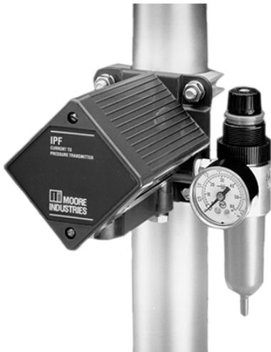
The rugged IPF Field-Mounted Current-to-Pressure Transmitter is designed specifically for installation in harsh environments. The two-wire IPF accepts a 4-20mA or 10-50mA input. It converts the input to a 3-15psig, 0.2-1bar, 15-3psig or 1-0.2bar pneumatic output signal, or to a wide variety of other commonly used pneumatic outputs and is available with an optional coalescing filter/regulator that combines both an air filter and a miniature supply line regulator.
