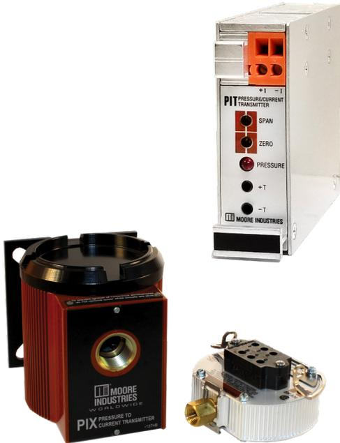
This rugged and reliable family of pressure-to-current transmitters provide an economical solution when a pneumatic device must interface with a data acquisition control system, controller, recorder, or other electronic instrument. Compact, yet powerful, these units accept a pneumatic signal (3-15 psig, 0.2-1 bar, 3-27 psig, etc.) and accurately convert it to a proportional 4-20mA (or 10-50mA) output.
