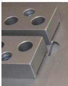
Figure 5: Notches between the pressure strip and back
