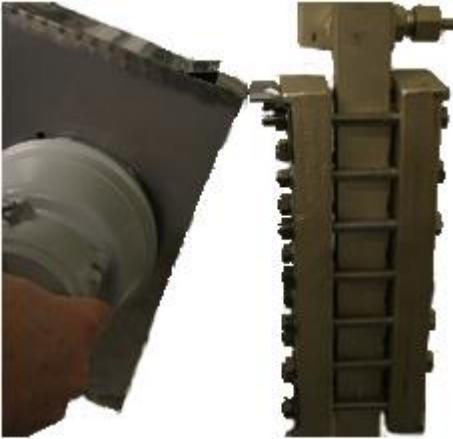
Now, the bent side of the light guide box can be hung on the corresponding mounting bracket.
