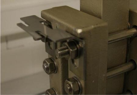
The illumination unit with halogen bulb is mounted using the mounting angle installed on the glass gauge.
