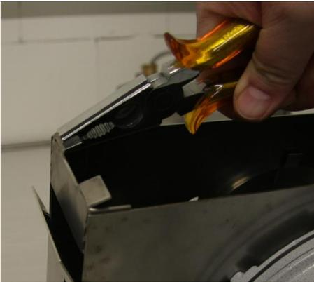
The illumination unit can be installed with the bulb casing to the right and left from the perspective of the viewing direction. Both of the arms on the mount on the upper side of the light box must be bent approx. 60°C using a pair of pliers.
