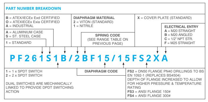
NOTE: RESISTORS ARE INDICATED BY THE PREFIX "PR" IN PLACE OF "PF".
