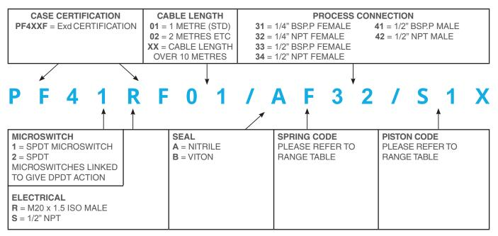
Certification: All switches are ATEX / IECEx certified for gas hazardous areas and are CE marked. Exd Flameproof: Ex II 2 G Ex db IIC Gb T6 Tamb -50 to +71°C, T5 +86°C, T4 +100°C Special conditions for safe use:
