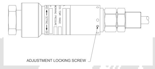
The design features a simple form of adjustment. This enables users to order switches set at a predetermined point or stock a mid range setting and adjust switches to suit the particular application. Rotating the outer tube compresses the discsprings. Rotation clockwise will increase the set point and conversely rotating anti-clockwise will decrease the set point.
