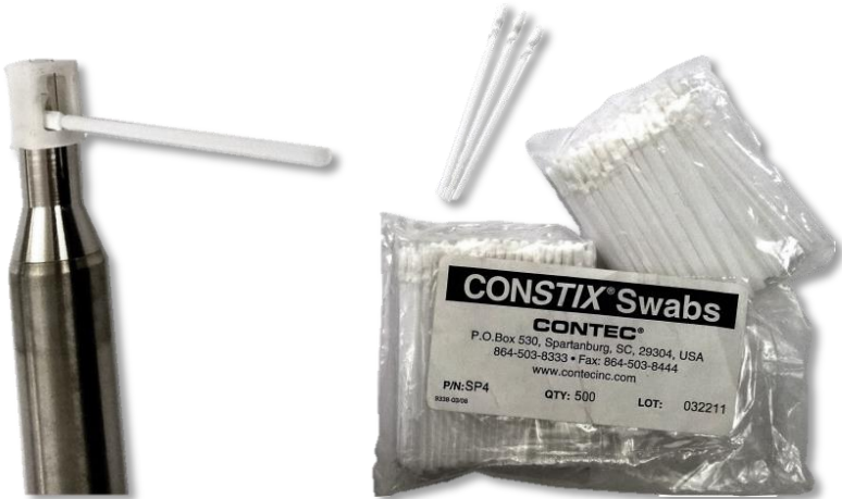
Figure 8-1 Suitable cotton swabs with small cleaning pads
