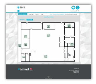
**Plan View** provides visual indication of sensor location within a facility. Sensor icons show real-time data and alarms and interaction by double clicking icon.
