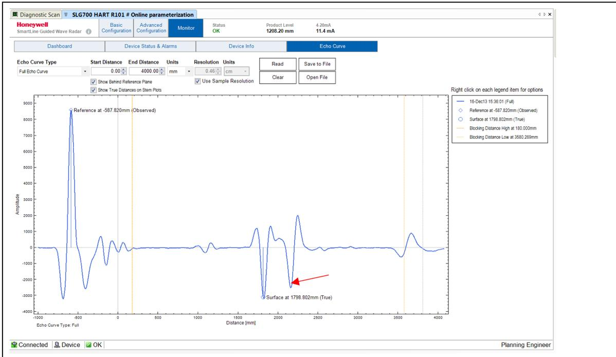
**Misplaced spacer:** The red arrow points to the position where the central conductor is likely touching the outer tube. The point of contact is ~2 m; however, since the level is higher than this position, the false reflection appears further away due to the index of refraction effect.
