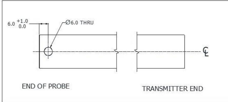
**Figure 5-14 - Drill Hole Position on Outer Tube**
