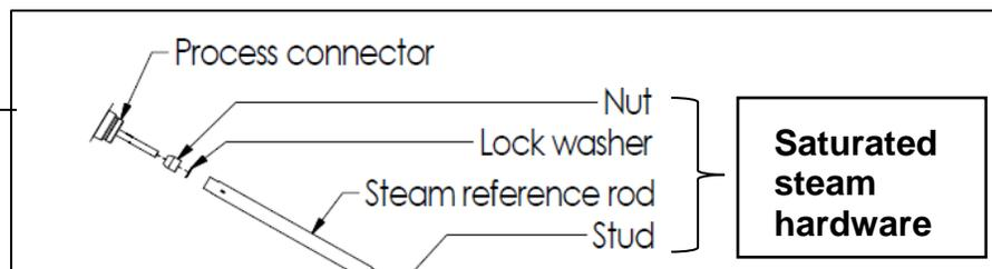
**Figure 3-15 Saturated steam application rod probe assembly**
