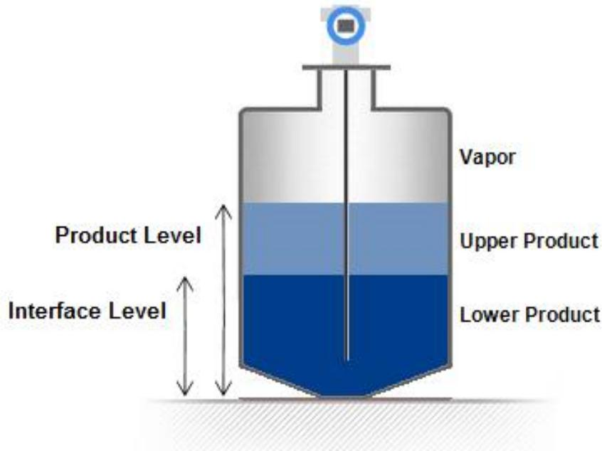
**Figure 2-3: Interface measurement**
