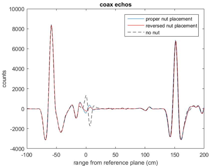
This illustrates the importance of proper nut placement. The biggest effect is from a nut missing altogether
