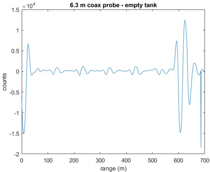
This illustrates a properly assembled coax probe with an empty tank. The spacers are visible on the probe every meter but their heights are small (<1000 counts). The large reflection at 6 m is the end of the probe.
