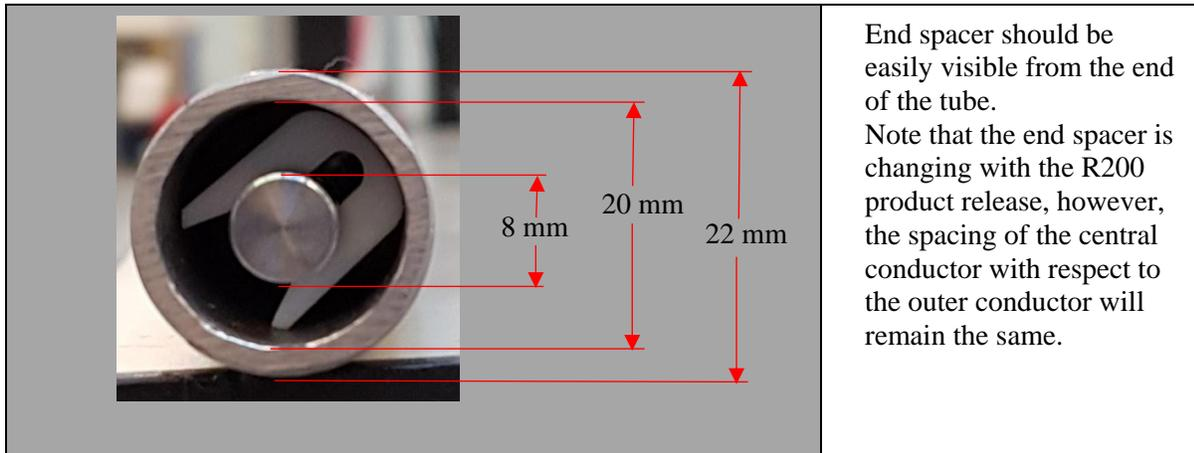
In some cases, the spacers may be jammed between the inner conductor and outer tube. If you suspect this might be the case, it is possible to diagnose by measuring from the outside of the tube to the central conductor using the depth gauge on a micrometer. The distance expected is  $(7\pm 2)$  mm.
