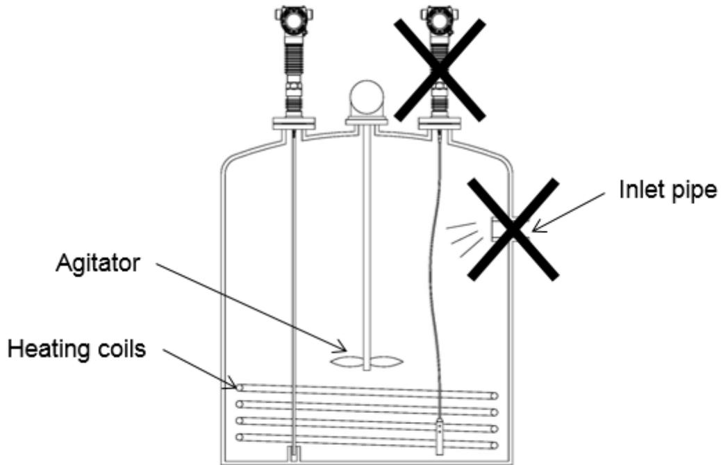
Figure 3-27: Mounting position
