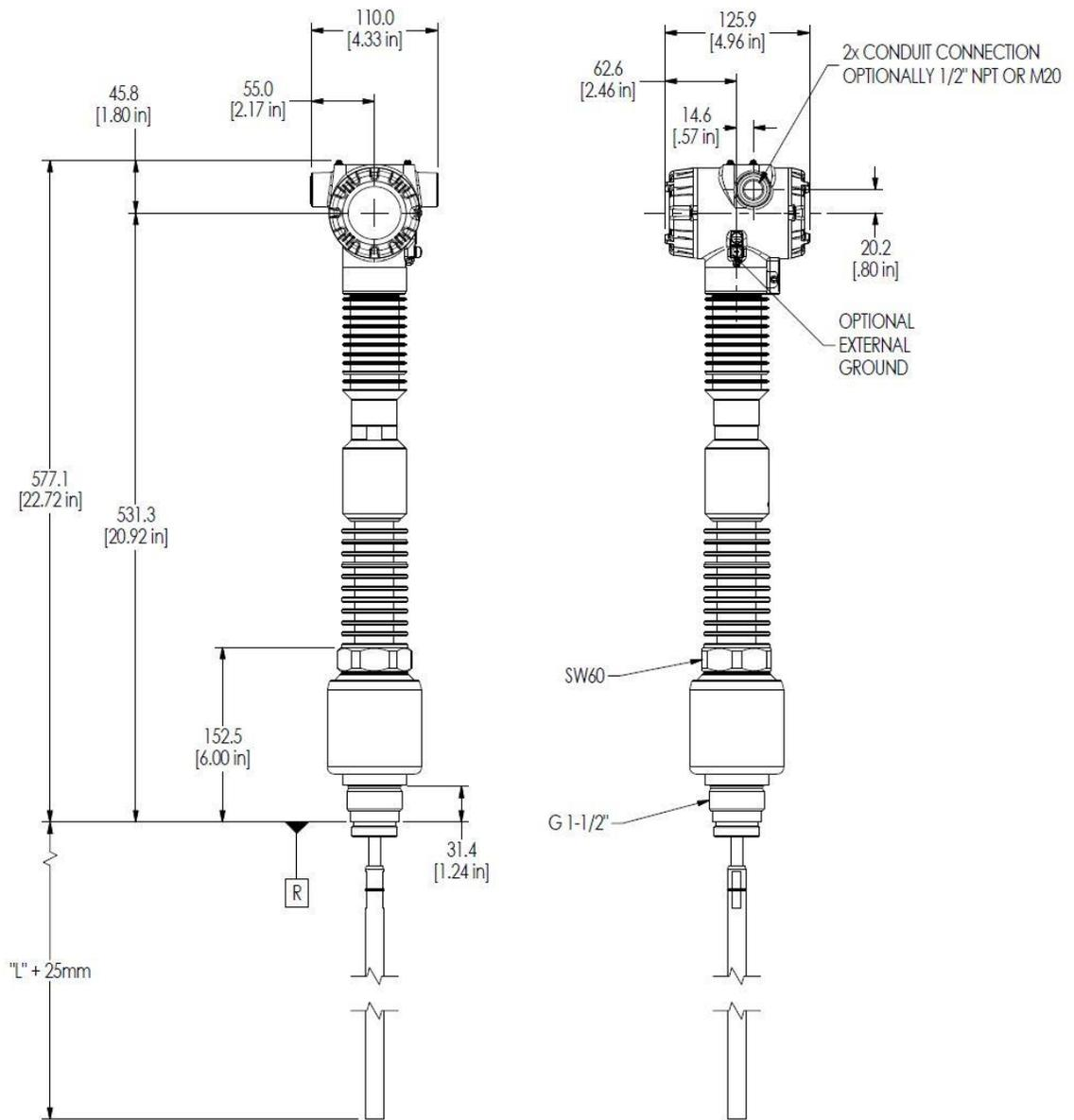
**Figure 3-26: Threaded (BSP/G 1½") SLG726 transmitter, mm [in]**
