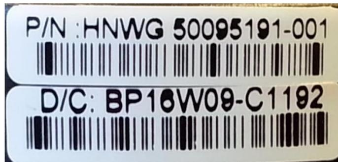
**Figure 5-45-5: Part Number and Date Code (D/C) label on bottom of Terminal PCBA**
