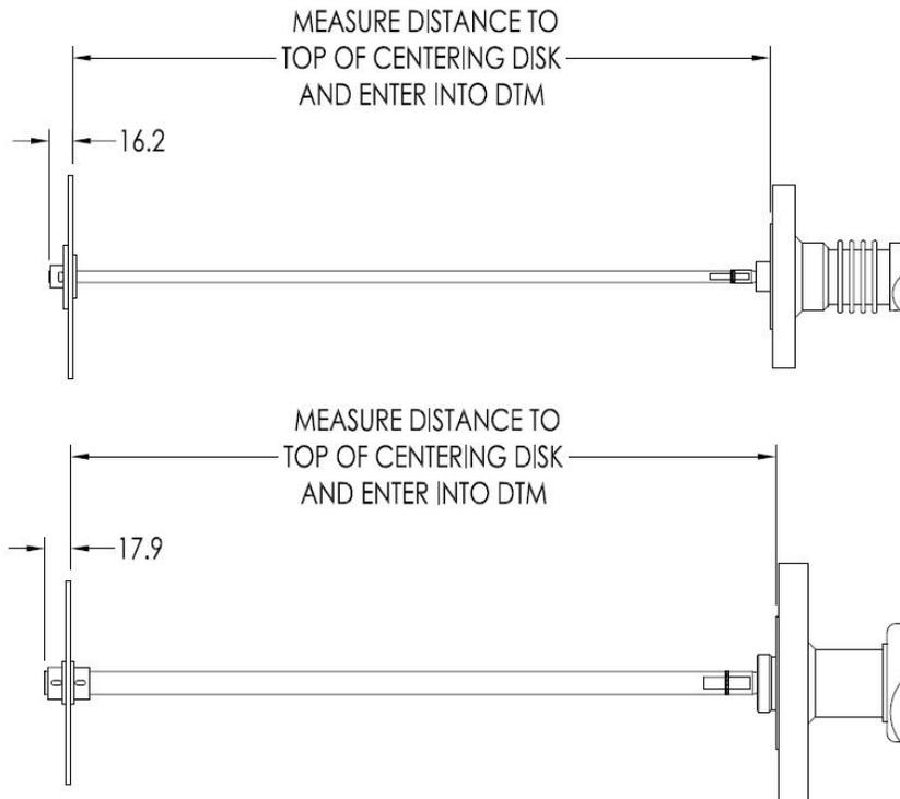
**Figure 3-20: Probe length definition for rod probes using a centering disk**
