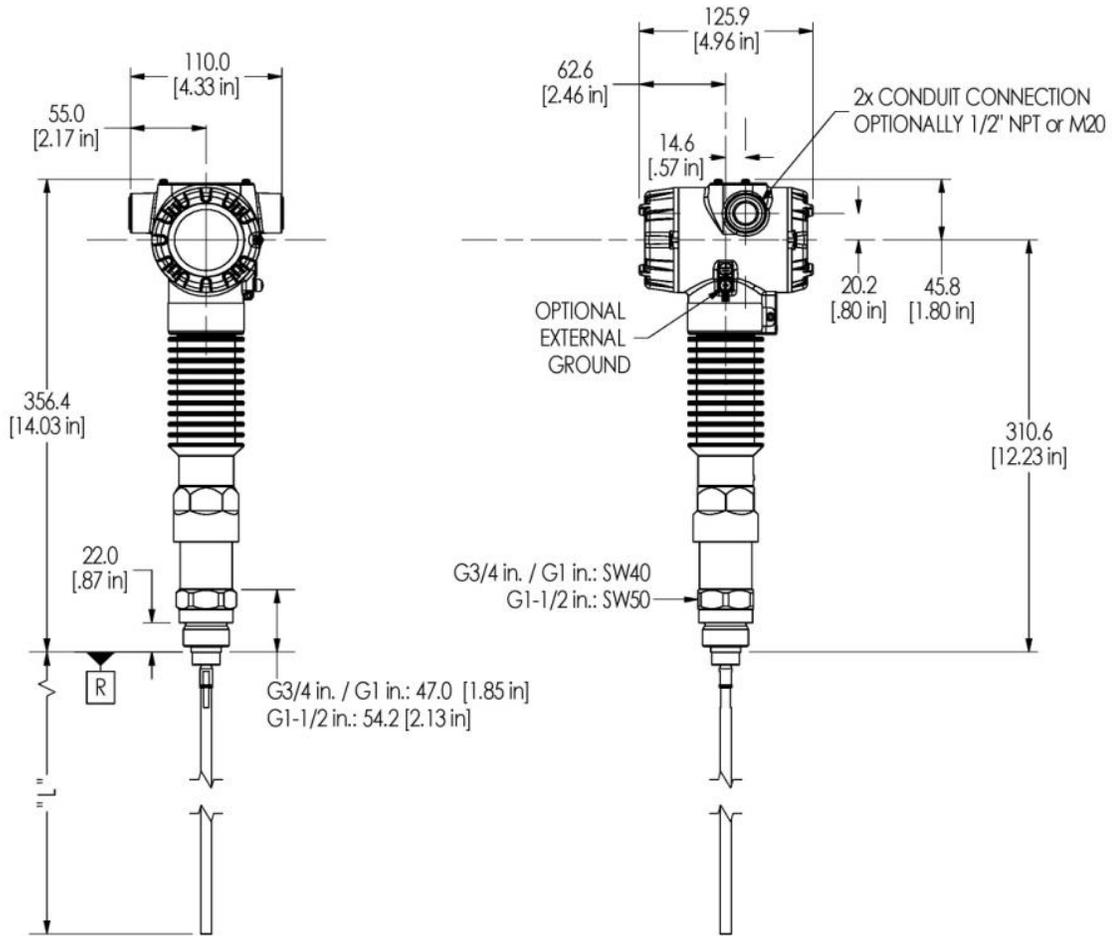
Figure 3-23: Threaded (BSP/G 3/4", 1", 1 1/2") SLG720 Transmitter, mm [in]
