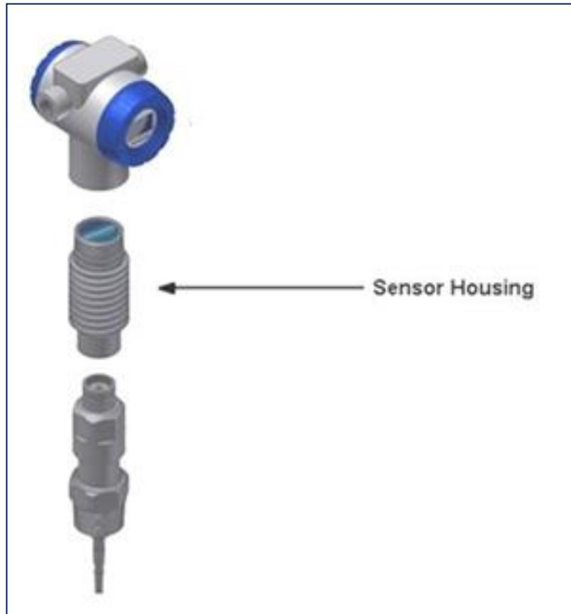
Figure 5-3: Sensor Housing
