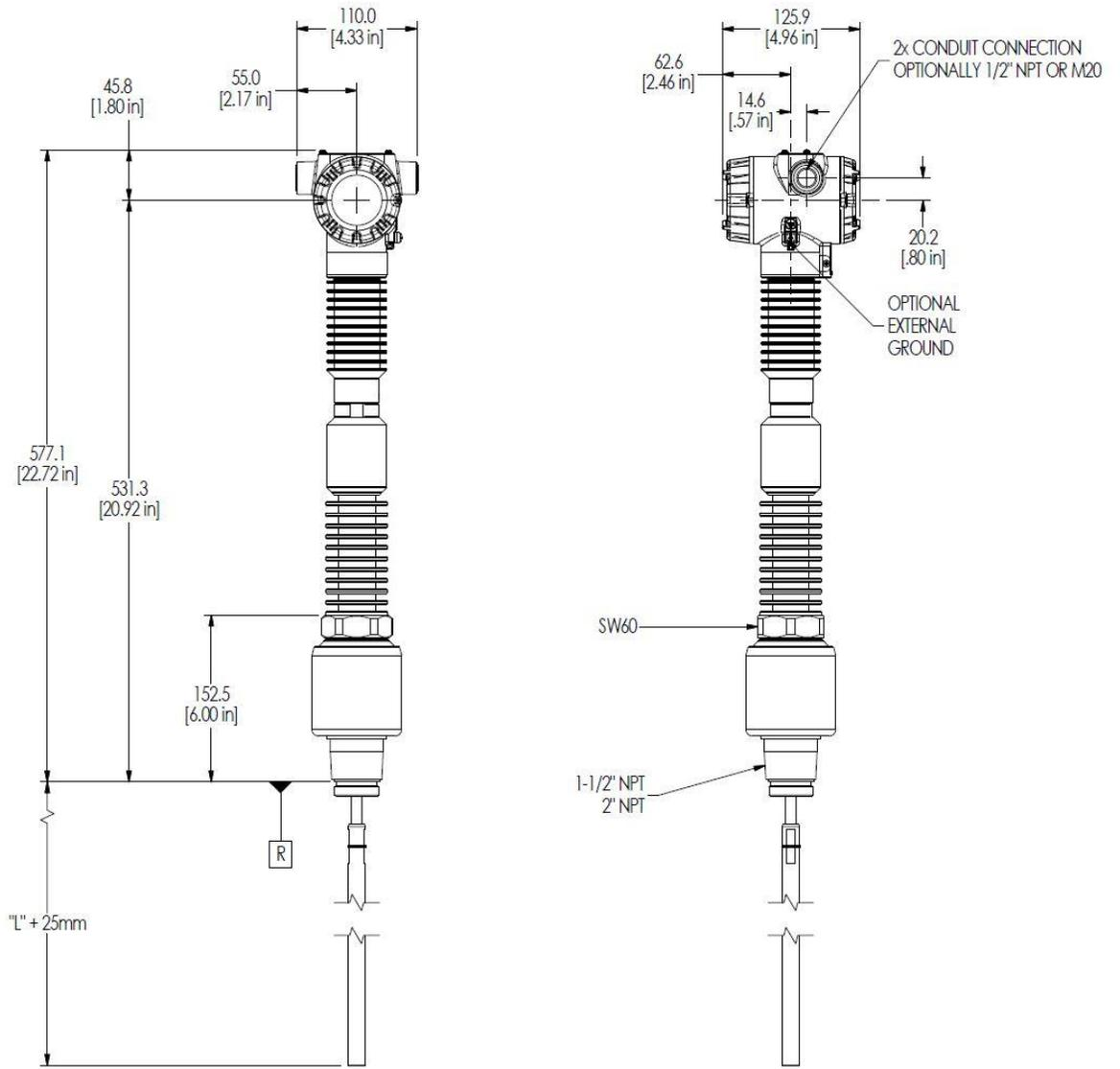
**Figure 3-25: Threaded (NPT 1½", 2") SLG726 transmitter, mm [in]**
