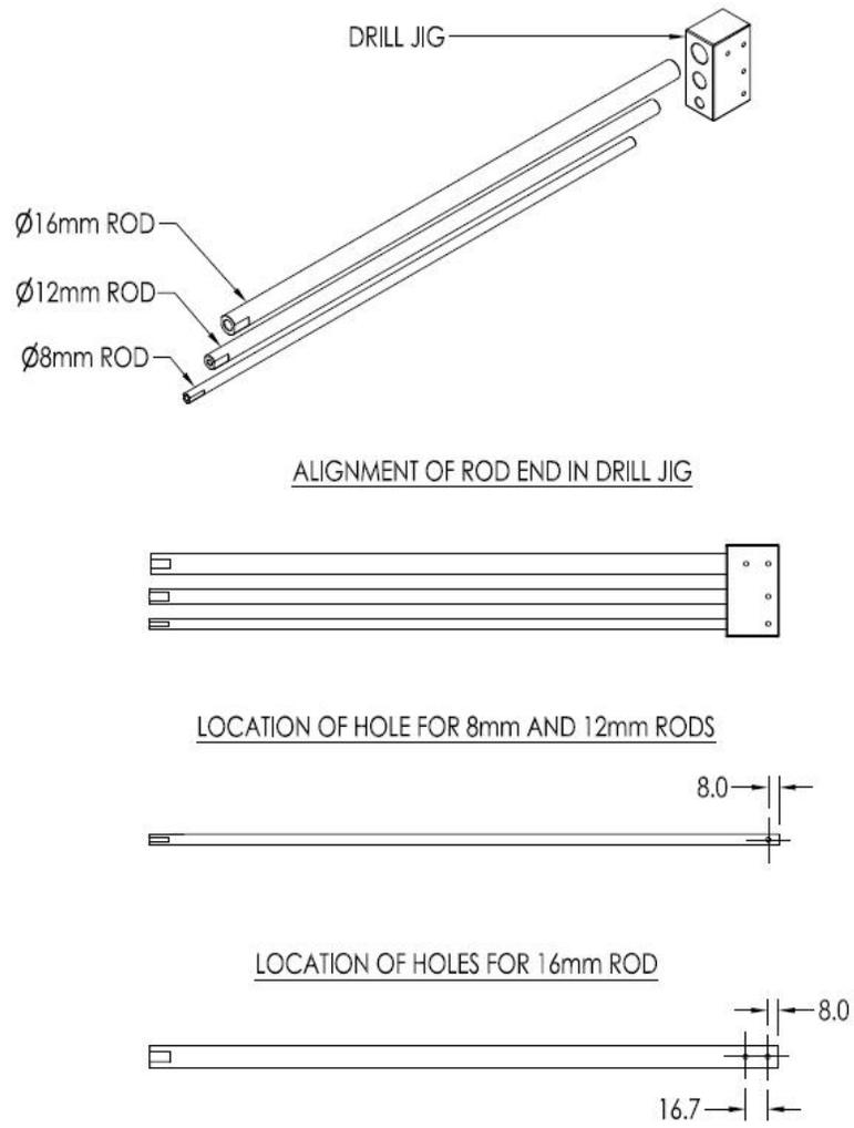
**Figure 3-17: Recommended location of holes for rod probes**
