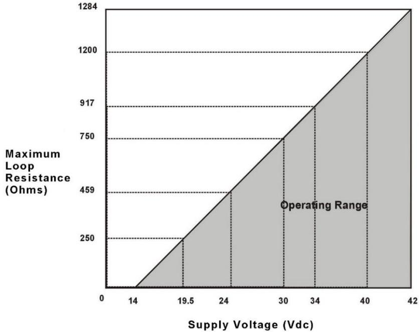
**Note: A minimum of 250ohms of loop resistance is required to support communications.**
