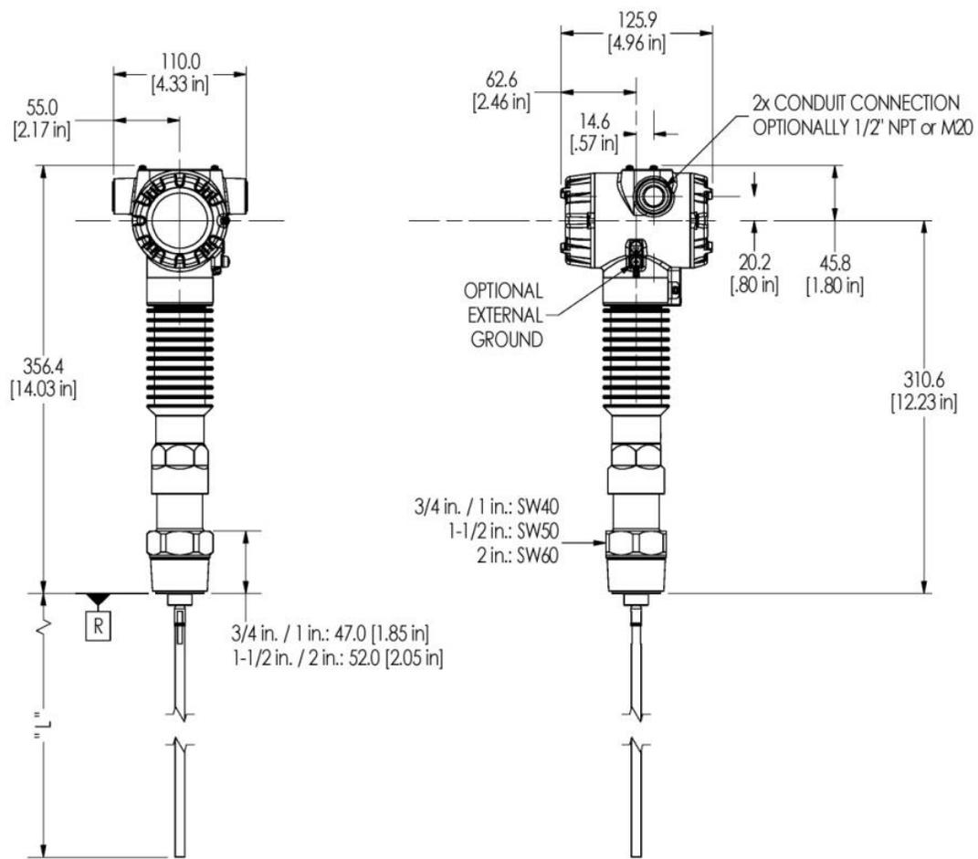
**Figure 3-22: Threaded (NPT 3/4", 1", 1½", 2") SLG720 Transmitter, mm [in]**
