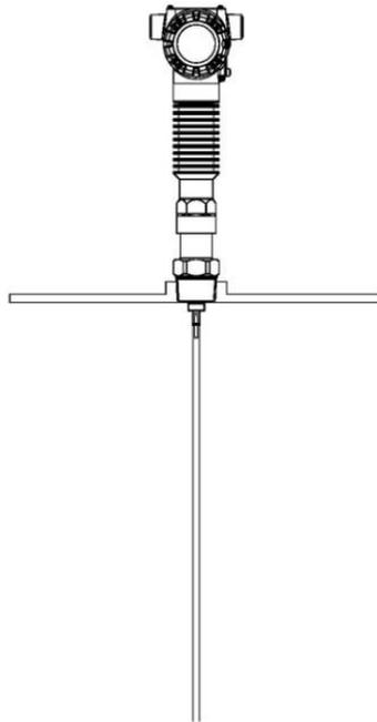
**Figure 3-35: Tank roof mounting using threaded connection**
