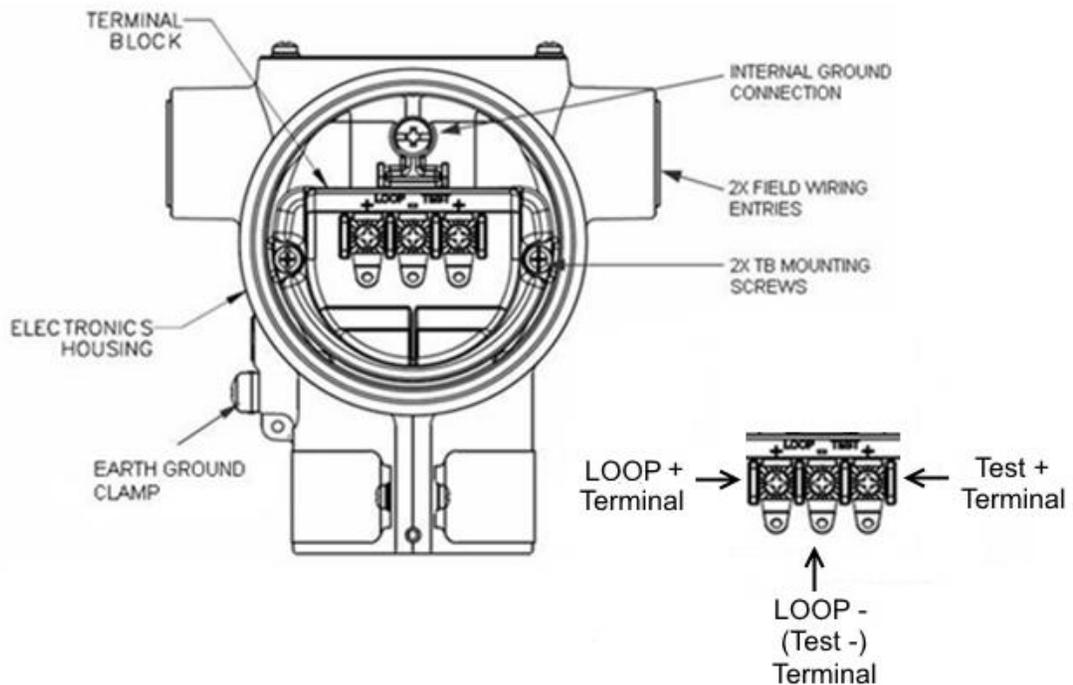
**Figure 3-45: HART 3-Screw Terminal Board and Grounding Screw**
