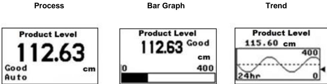
Figure 4-2: Advanced Display Formats with the Process Variable
