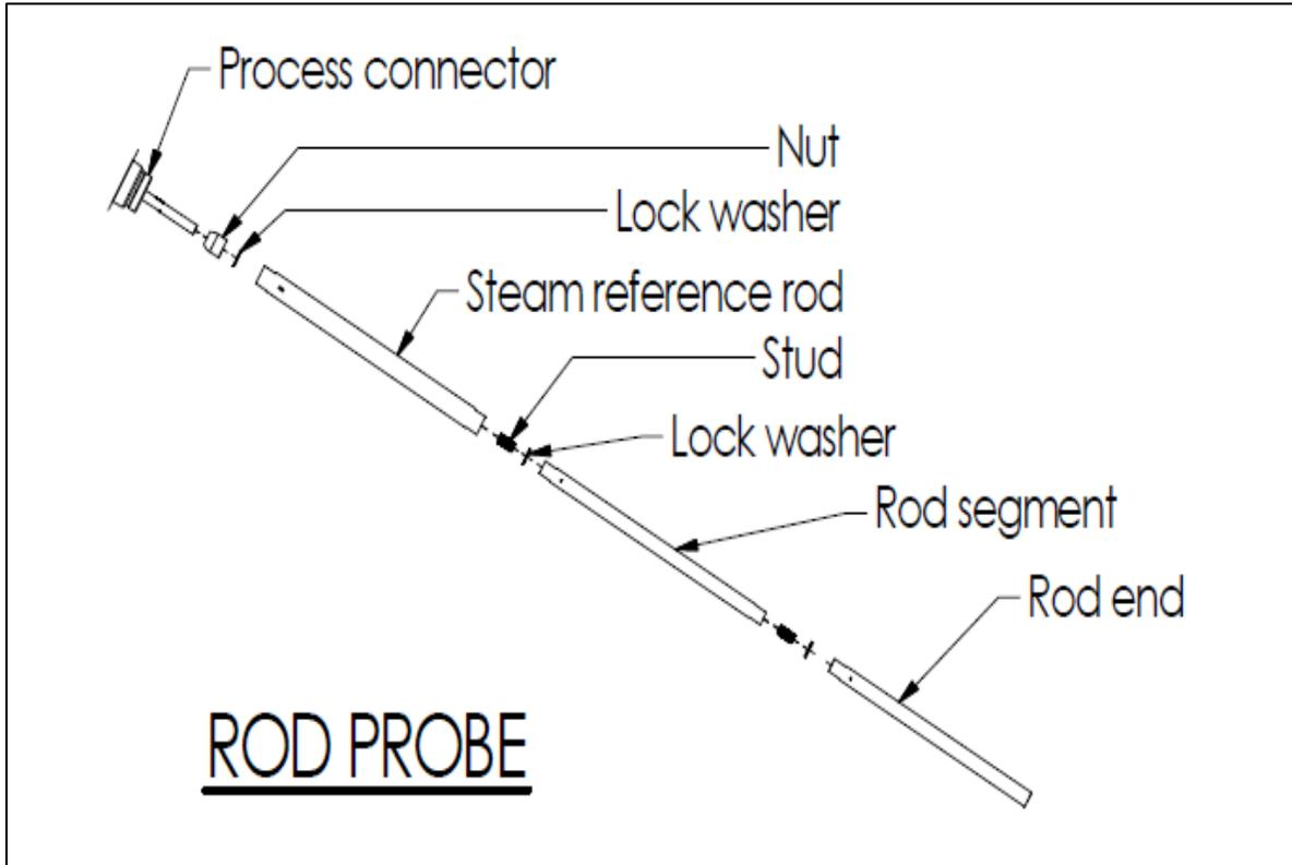
**Figure 5-17 - Saturated steam application rod probe assembly**
