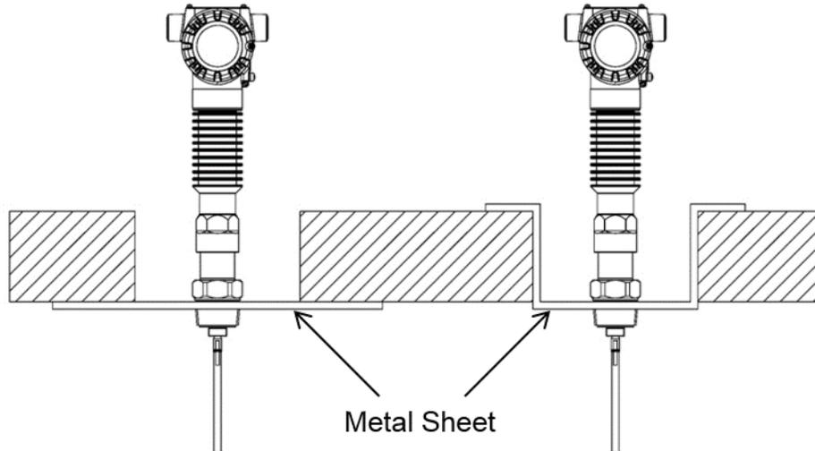
**Figure 3-38: Mounting in concrete silos**
