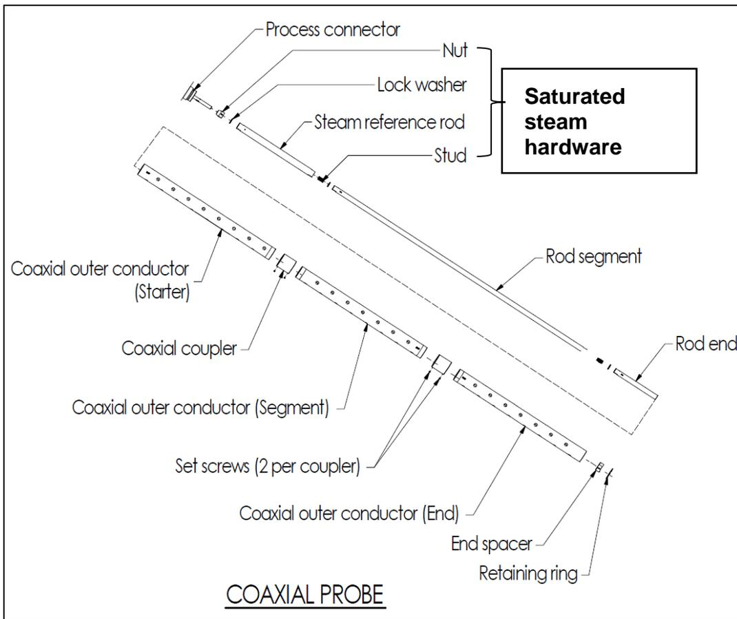
**Figure 3-16: Saturated steam application coaxial probe assembly**
