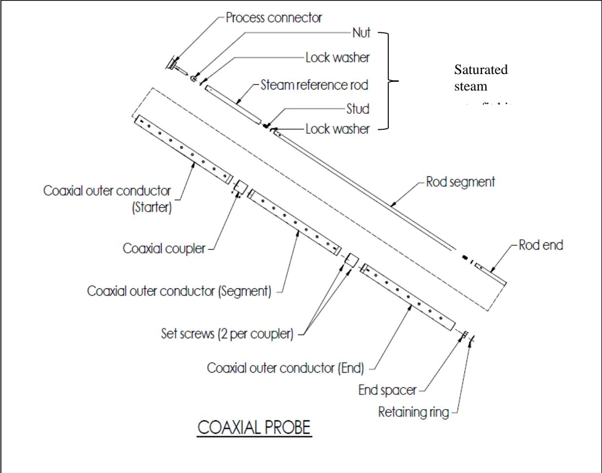
**Figure 5-18 - Saturated steam application coaxial probe assembly**
