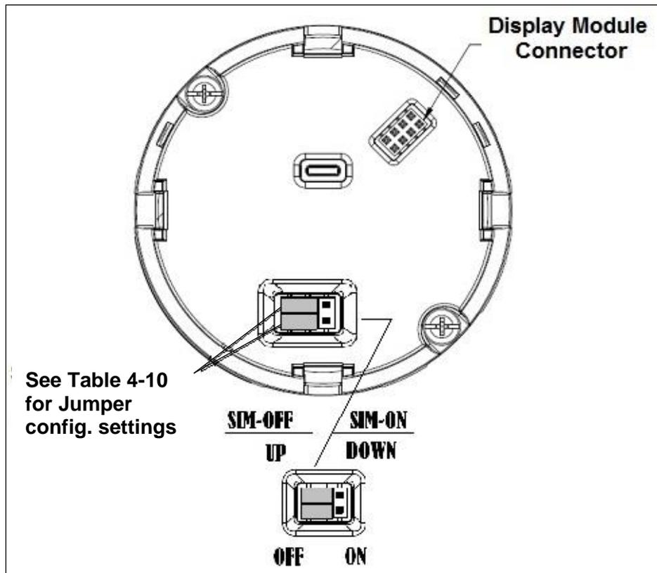
**Figure 4-3: Locating the Failsafe and Write Protect Jumpers**
