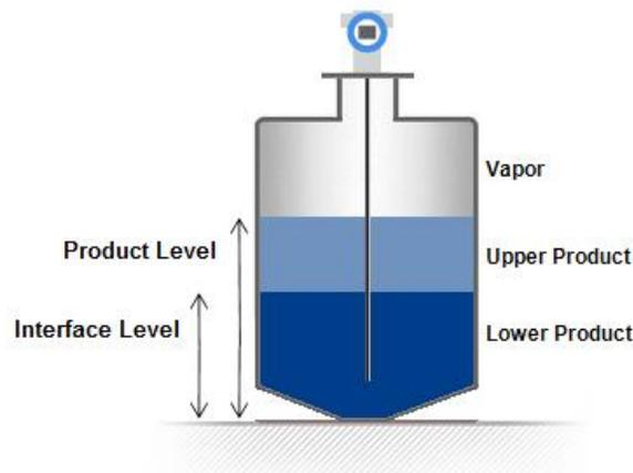
**Figure 2-12: Two-liquids non-flooded.**
