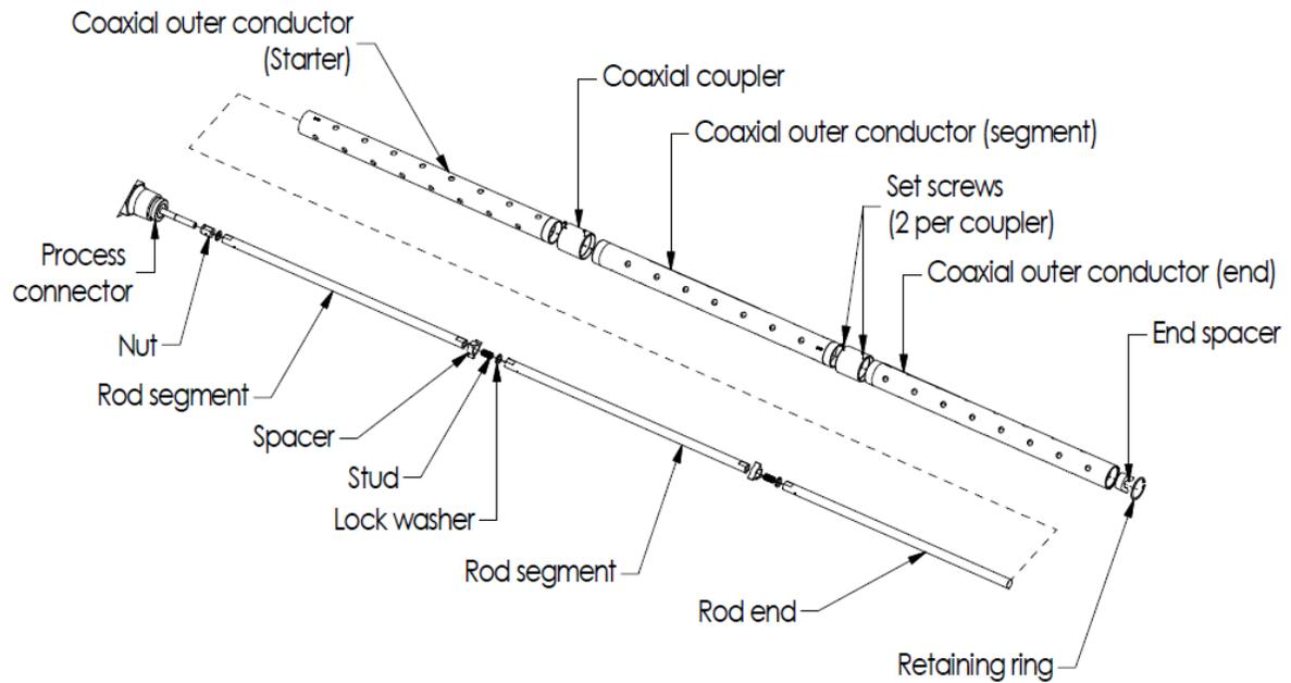
**Figure 3-14: SLG726 Coaxial probe assembly**
