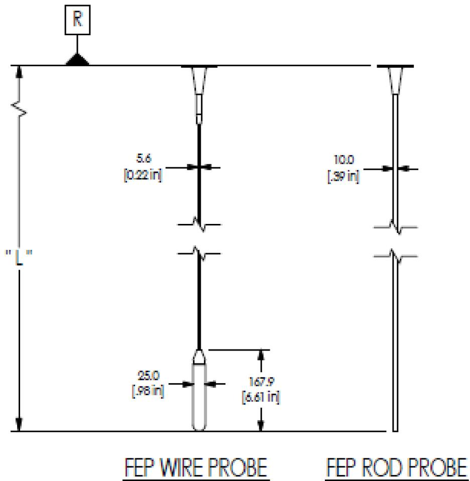
Figure 3-2: SLG720 FEP probe dimensions, mm [in]
