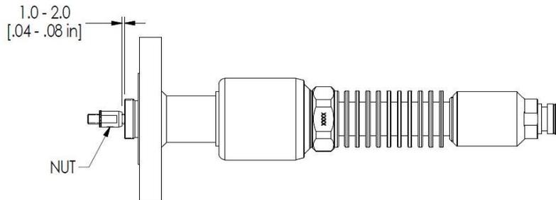
If the probe length has changed measure the length from the reference plane to the end of the probe. **Keep in mind that for a wire probe with an end weight, the probe length is measured from the transmitter reference plane to the top of the end weight.** If the wire probe is untrimmed, it is possible to determine the correct probe length from the factory by following these steps:
