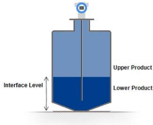
**Figure 2-11: Two-liquids Flooded**
