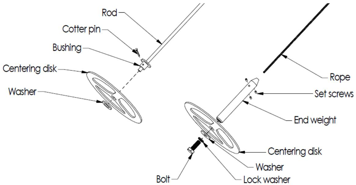
**Figure 3-18: Centering disks for wire and rod probes.**
