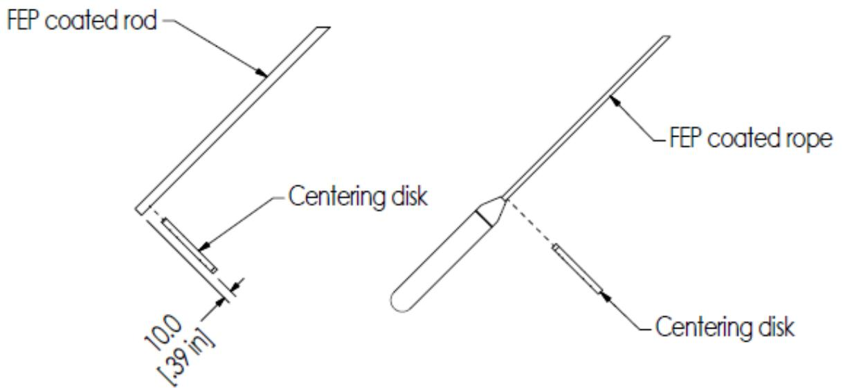
**Figure 3-19: Centering disks for FEP coated wire and rod probes**
