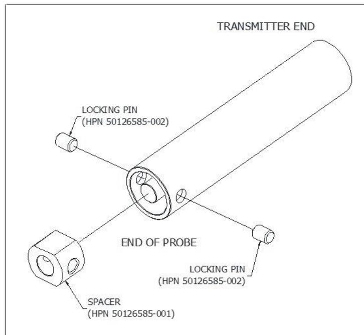
**Figure 5-15 - Spacer and Locking Pin Installation**
