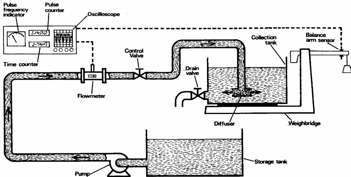
Water is pumped from storage through the test meter, through a manual control valve into a collecting tank mounted upon a standard weighbridge, the vessel having a drain valve for return to storage. At the commencement of a calibration, water is circulated through the system and allowed to drain whilst the operator regulates the control valve to set up the approximate desired flowrate.
