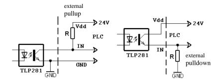
The maximum frequency of the impulse output is 900Hz with min. 250µs pulse width.
