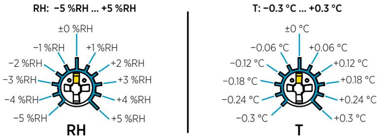
Figure 6 RH and T Trimmer Adjustment Ranges (Indicative)
