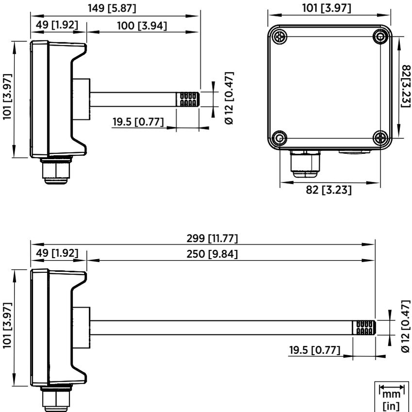
Figure 27 Dimensions with Long and Short Probe
