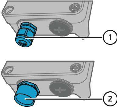
**Figure 2** HMD60 Cable Gland and Conduit Options
