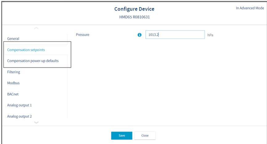
Figure 16 Pressure Compensation Settings
