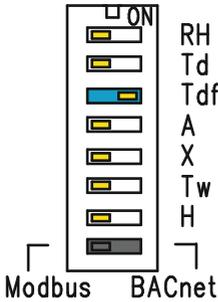
Figure 7 HMD65 DIP Switch Example:  $T_{df}$  Output Selected
