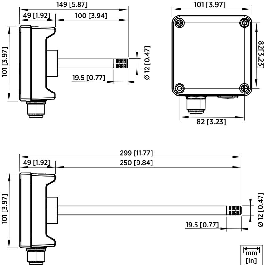
Figure 8 Dimensions with Long and Short Probe
