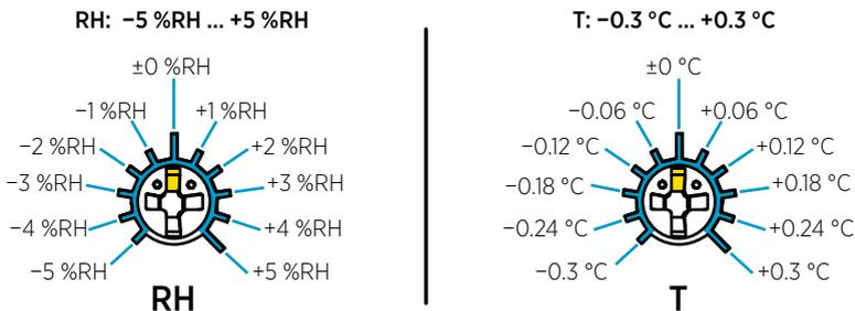
Figure 25 RH and T Adjustment Trimmer Ranges (Indicative)
