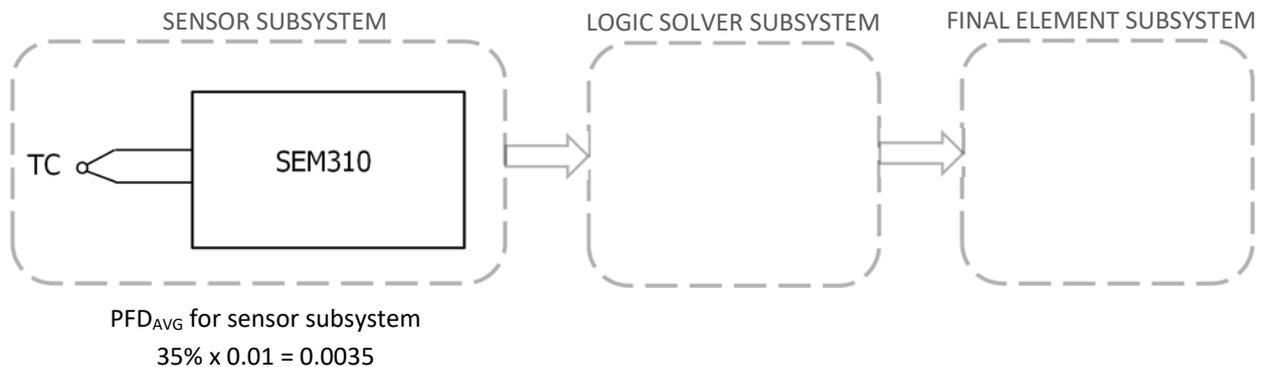
For the purposes of illustration only, example TC failure data is shown, together with the FMEA failure data for the SEM310 from page 1. (Note that failure data quantities are summed to get the corresponding parameter value for the sensor subsystem).
