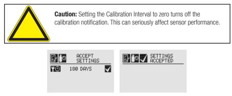
Figure 108. Saving New Interval and New Interval Accepted Screens
