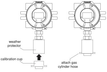
Figure 203. Attaching the Calibration Cup
