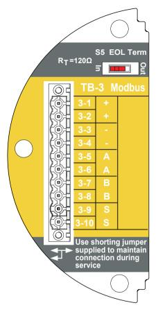
Figure 248. Modbus connections
