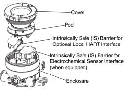
Figure 2. XNX Exploded View
