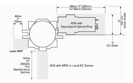
Figure 24. XNX Universal Transmitter mounting dimensions and clearances
