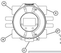
While relay wiring can use any available cable/conduit port in the XNX enclosure, do not use the same cable/conduit port for both relay reset and relay signal lines to avoid electrical noise.
