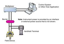
Figure 233. HART Point-to-point Mode
