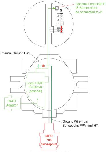
Figure 46. mV Personality Wiring
