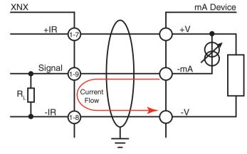
Figure 50. XNX mA input source configuration
