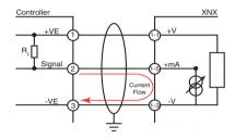
Figure 36. Sink wiring for XNX
