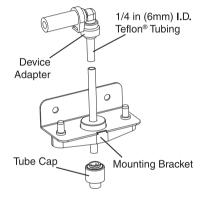
The Remote Gassing Kit (1226A0354) enables gas to be applied remotely for performing functional response checks (bump tests). The kit Includes: 50' Teflon<sup>®</sup> tubing, a mounting bracket, a tube cap, and device adapters in 1/4" and 1/8" (6.3 mm and 3.2 mm) ID to attach to bump test ports on the weatherproof cap of the device.
