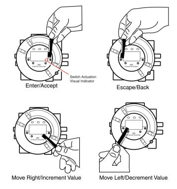
Figure 9. Using the magnetic wand
