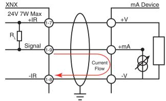
Figure 49. XNX mA input sink configuration
