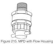
4. Connect the flow housing (using either gas pipe) to the regulated cylinder containing a known concentration of the target gas at approximately the sensor alarm point, e.g., 50% LEL methane in air.
