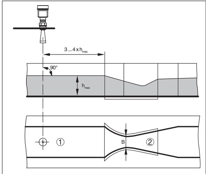
Fig. 22: Flow measurement with Khafagi-Venturi flume:  $h_{max}$  = max. filling of the flume; B = tightest constriction in the flume
