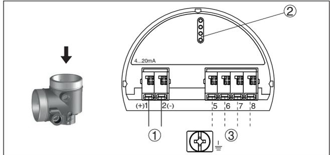
Fig. 28: Electronics compartment - Ex-d-ia double chamber housing
