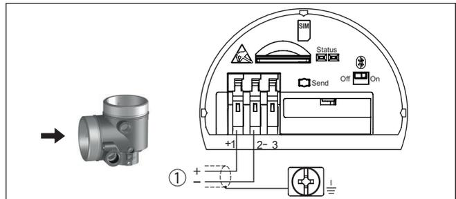
Fig. 27: Connection compartment - Radio module PLICSMOBILE 81
