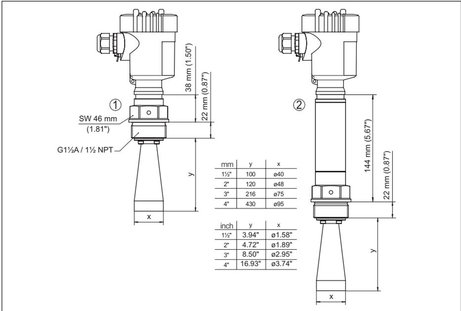
Fig. 64: VEGAPULS 62, horn antenna in threaded version
