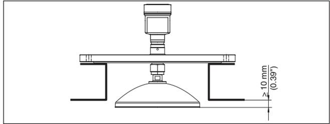
Fig. 9: Recommended socket mounting with parabolic antenna
