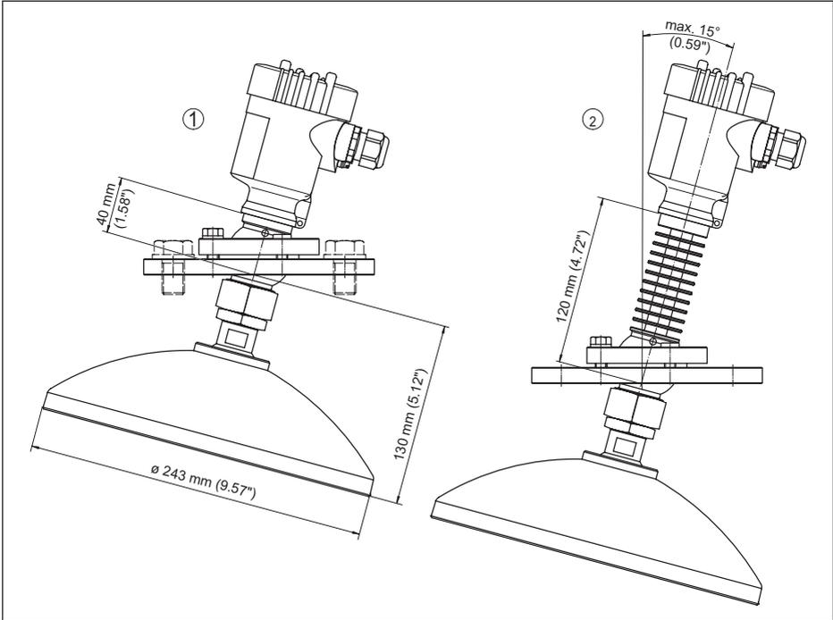
Fig. 70: VEGAPULS 62, parabolic antenna and swivelling holder
