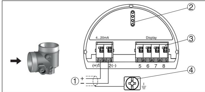
Fig. 26: Connection compartment - double chamber housing
