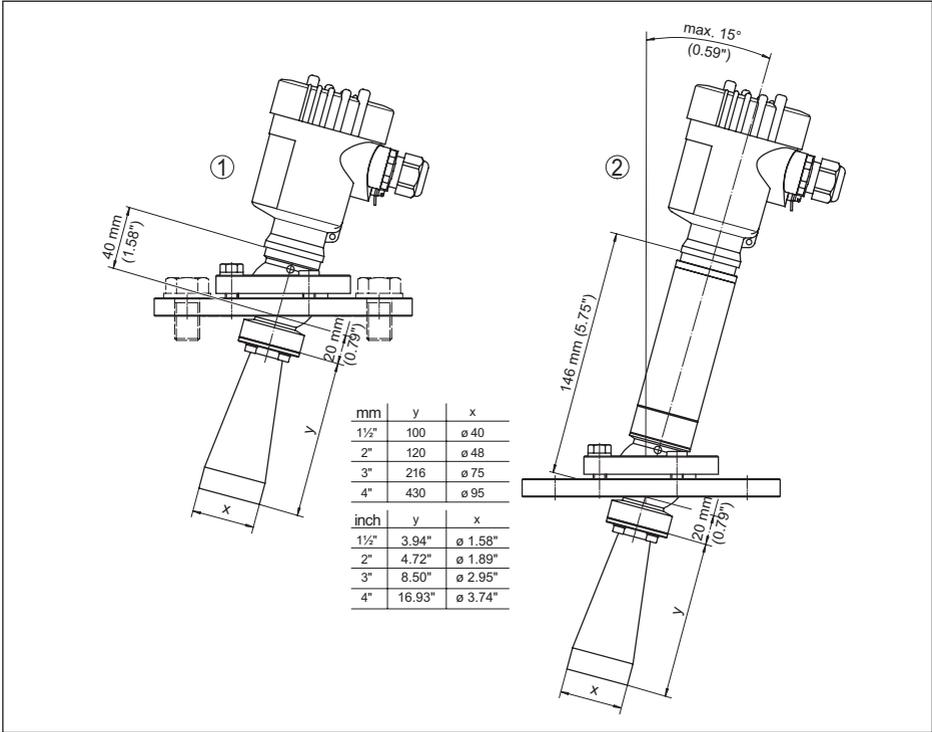
Fig. 68: VEGAPULS 62, horn antenna and swivelling holder
