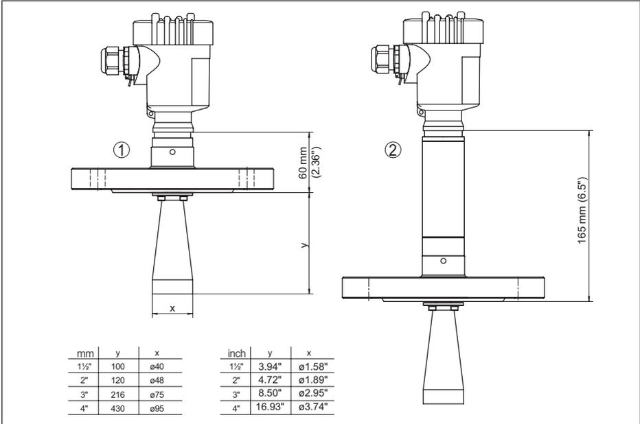
Fig. 65: VEGAPULS 62, horn antenna in flange version
