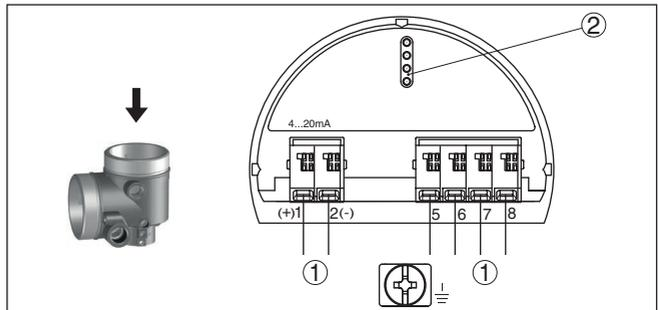
Fig. 25: Electronics compartment - double chamber housing
