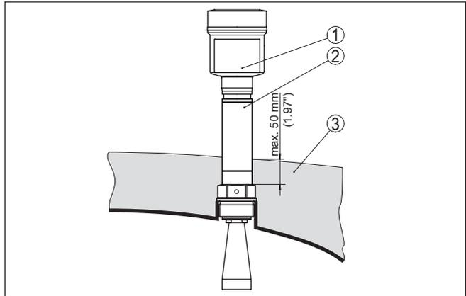
Fig. 17: Mounting the instrument on insulated vessels.
