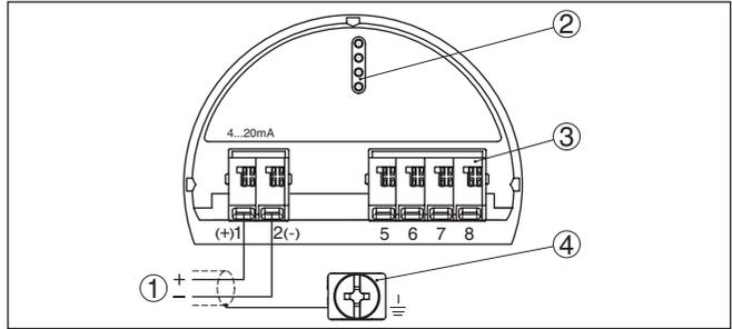
Fig. 24: Electronics and connection compartment - single chamber housing
