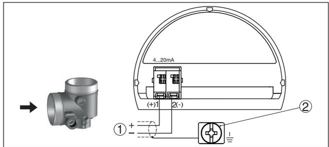
Fig. 29: Connection compartment - Ex-d-ia double chamber housing
