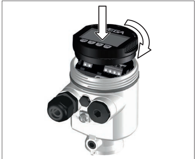
Fig. 28: Installing the display and adjustment module in the electronics compartment of the single chamber housing
