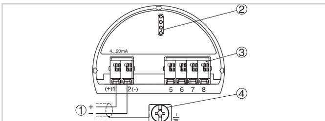
Electronics and terminal compartment, single chamber housing
