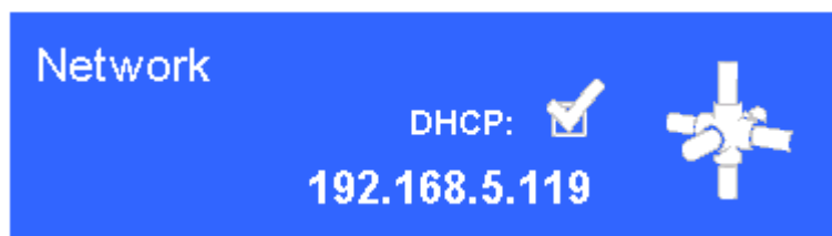
Fig. 5-1 The IP address of the Q.monixx with DHCP enabled, as seen on the Q.monixx A117 D LCD display
