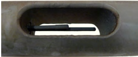
Example of Dirty Sensor
