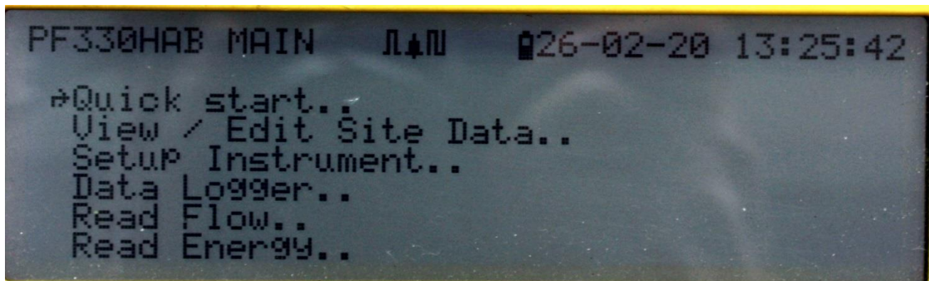
Figure 6 Main menu ( Read Energy and Data Logger options available with 333 models only )
