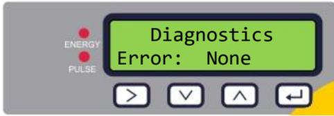
This screen will display the Errors. A number between 0-255 will be displayed. If no errors reported "None" is displayed.
