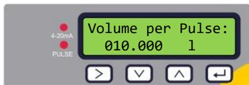
Set the Volume per Pulse so that the maximum number of pulses does not exceed 10 per second or 1000ms (see page 26).
