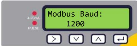
Enter the baud rate for the Modbus network. Valid settings are 1200, 2400, 4800, 9600, 19200, or 38400.
