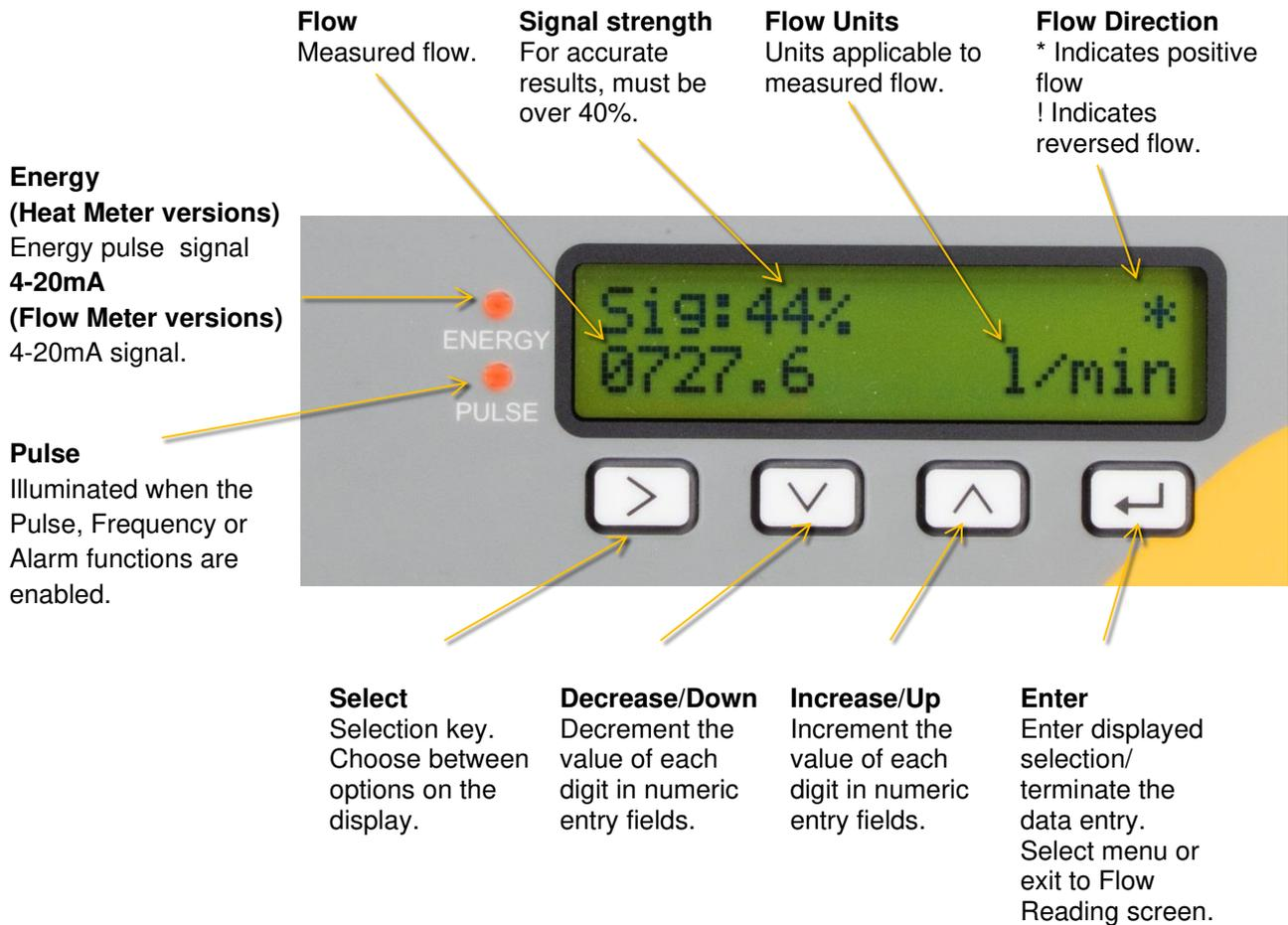
**Figure 3 U1000MKII WM display (Heat Meter model shown)**
