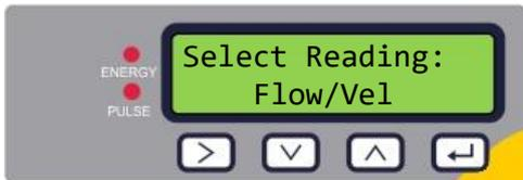
Choose the default display option: *Flow* (flow rate, for example, l/min) or *Vel* (velocity, for example, m/s).
