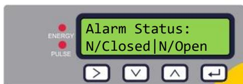
Select the status of the pulse output during normal operation: **Normally Closed** or **Normally Open**.
