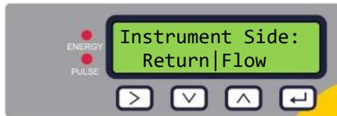
Select the Instrument Side (where flow sensors are installed) using
