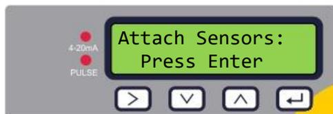
You are prompted to attach the sensors. Place the PT100 sensors touching each other and allow their temperature to stabilise for 1 minute.
