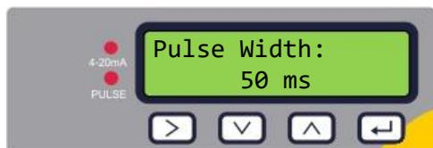
Set the Pulse Width. The default value is 50ms which represents half of one pulse cycle. A 50ms pulse width is required for most mechanical counters.
