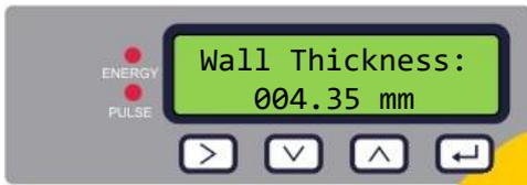
Enter the wall thickness of the pipe:
