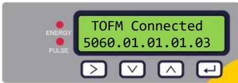
The flow board's firmware version is shown on the lower line. The upper line shows its status.
