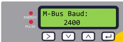
Enter the M-Bus Baud rate for this unit. The valid options are 300, 2400 or 9600 Baud.
