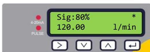
If a valid signal is found, signal strength and flow rate are displayed. The signal strength should be at least 40% for reliable operation.
