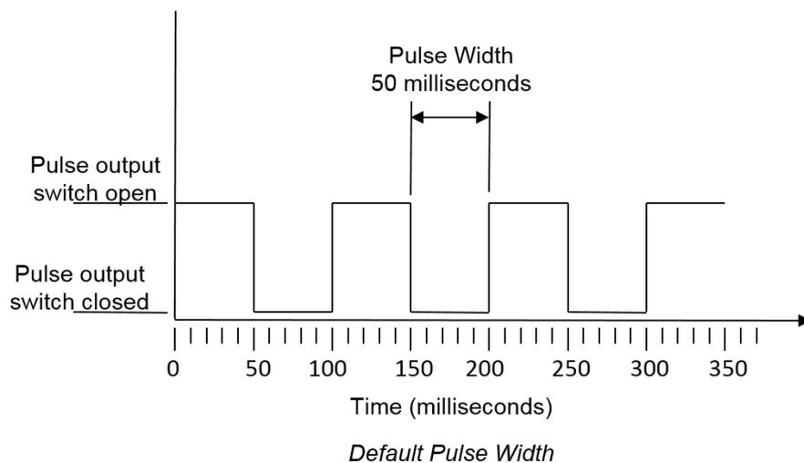
Formula to obtain Volume per Pulse based on a (default) 50ms pulse width:
