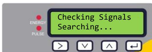
The unit checks for a valid flow signal.
