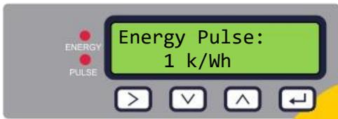
Choose from 1,10,100kWh or 1MWh when in metric mode and 1,10,100kBTU or 1MBTU in imperial mode. Each pulse represents the selected amount of energy e.g. 1kWh. Choose a value so that the pulse rate does not exceed 10 per second (see page 27).
