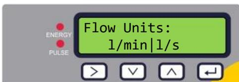
Choose the **Flow Units**. If you selected **mm** in the first step (*Select Dims*), the choice is l/min or l/s. If you selected **Inches**, the choice is gal/min or gal/hr (with either Imperial or US gallons according to the *System Units* selection).
