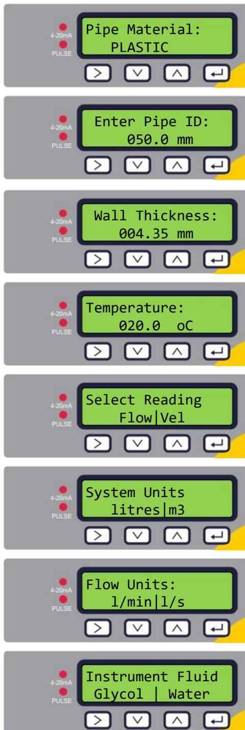
Select the pipe material by using the  $\uparrow$  and  $\downarrow$  keys to scroll through the list.
