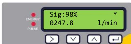
If a valid signal is found, signal strength and flow rate are displayed. The signal strength should be at least 40% for reliable operation.
