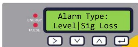
Choose the type of alarm: **Level**, triggering at a lowest acceptable flow rate, or **Signal Loss**, indicating a loss or malfunction of flow or signal.
