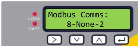
Select the Modbus data format. Valid settings are 8-None-2, 8-Even-1, 8-Odd-1, 8-None-1. The settings relate to the number of data bits in each character (8), the parity (Odd, Even or none), and the number of stop bits (1 or 2).
