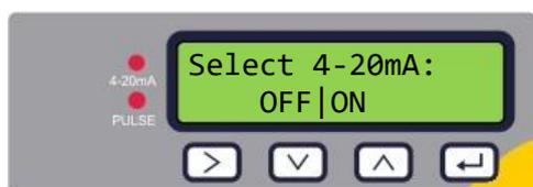
Enable or disable the 4-20mA output using
