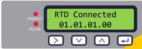
The RTD board's firmware version is shown on the lower line. The upper line shows its status.
