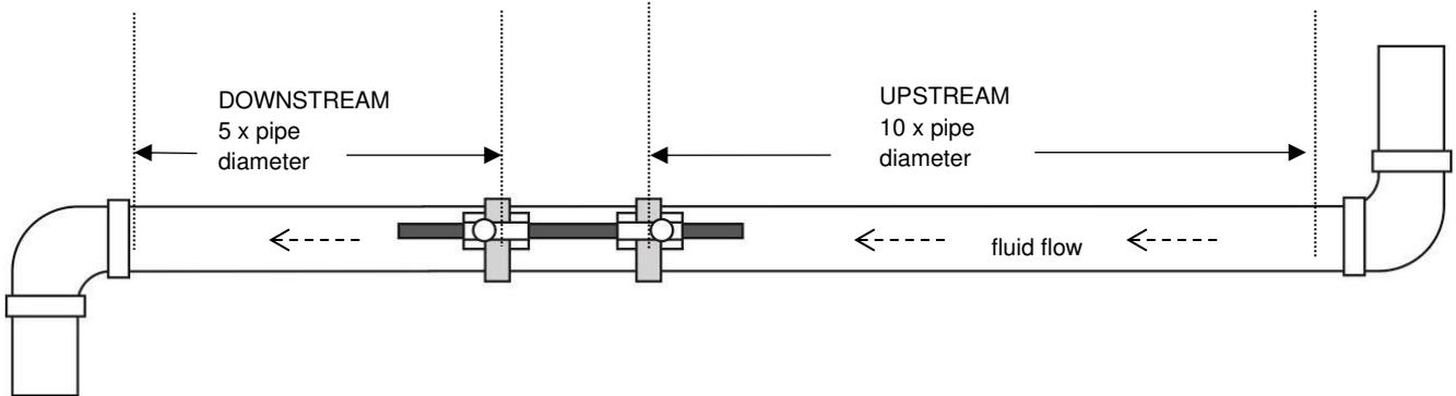
**Figure 4** Identifying a suitable location
