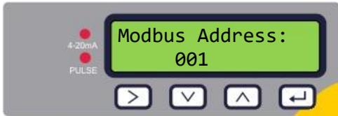
Enter the Modbus Address for this unit. The valid range is 1 to 126.
