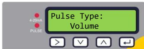
Choose the Pulse type: Volume, Flow Alarm, Energy (Heat Meter versions only), or Frequency.
