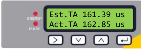
The Estimated TA (Time of Arrival) and Actual TA show the theoretical and measured transit times. If the actual value is displayed as 9999.99 then a usable signal could not be detected..
