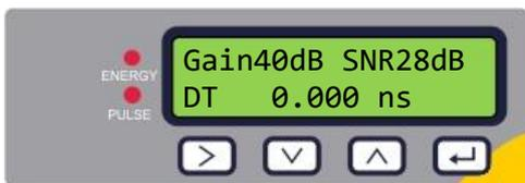
Gain – a decibel number between -5dB and 80dB – *lower is better*, should be around 40dB or below. Above 60dB need to question the installation.
