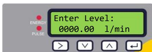
Only displayed if *Level* Type alarm type has been selected. Enter the flow value required to trigger the alarm.
