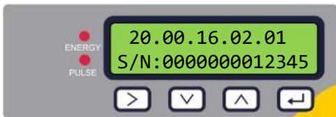
The unit's firmware version is shown on the upper line. The lower line shows the unit's serial number.
