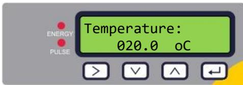
Enter the temperature of the fluid. The value must be in the range 0.1 – 140.0°C.
