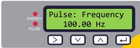
Displays the pulse status (for example): Deactivated, Volume 0.000 litres, Signal Loss, Alarm(On) 500.0 l/min, Alarm(Off) Signal Loss, Frequency 100.00 Hz.
