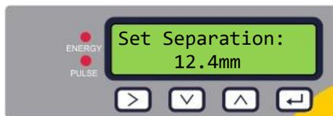
The unit now shows the correct flow sensor separation (in this case, "12.4mm") for the chosen values of pipe ID, pipe material and fluid.
