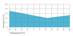
HMP1 temperature measurement accuracy over full range
