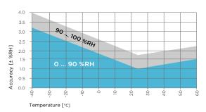
HMP1 humidity measurement accuracy as a function of temperature
