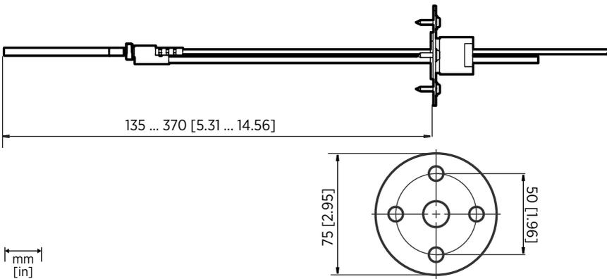
Figure 59 Optional duct kit 215003 dimensions
