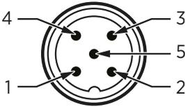
Figure 4 M12 5-pin A-coded male connector pinout
