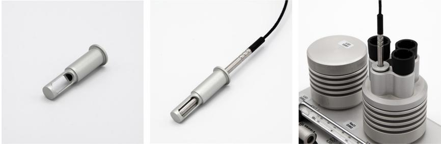
Figure 31 Using HMP9 calibration adapter with HMK15
