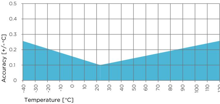
Figure 53 HMP9 temperature measurement accuracy over full range
