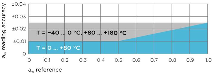
Figure 55 MMP8 A<sub>w</sub> measurement accuracy
