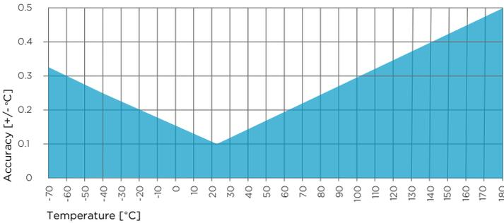
Figure 57 TMP1 temperature measurement accuracy over full range
