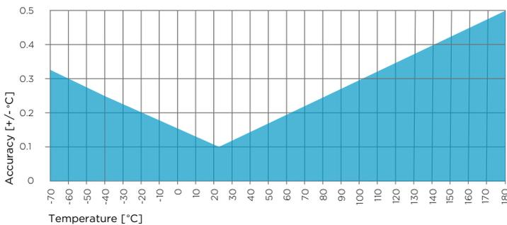
Figure 40 HMP4 temperature measurement accuracy over full range
