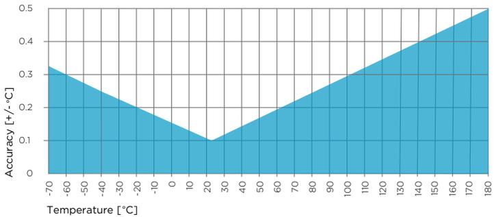
Figure 43 HMP5 temperature measurement accuracy over full range
