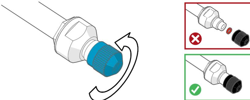
2. Push the probe head of HMP9 firmly through the sealing gland. Push the probe head further using its cable until it appears from the end of the tube. Adjust so that half of the metal probe head is visible, and tighten the sealing gland by hand so that it holds the probe cable in place.
