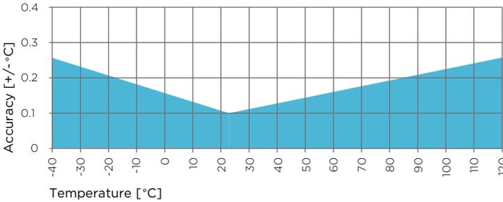
Figure 37 HMP3 temperature measurement accuracy over full range
