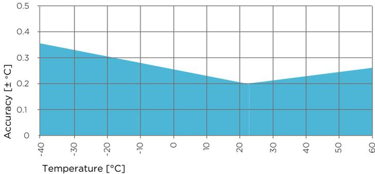
Figure 34 HMP1 temperature measurement accuracy over full range
