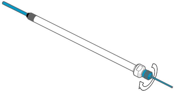
3. Insert the mounting flange on the pipe. Make sure the black sealing surface faces the probe head.
