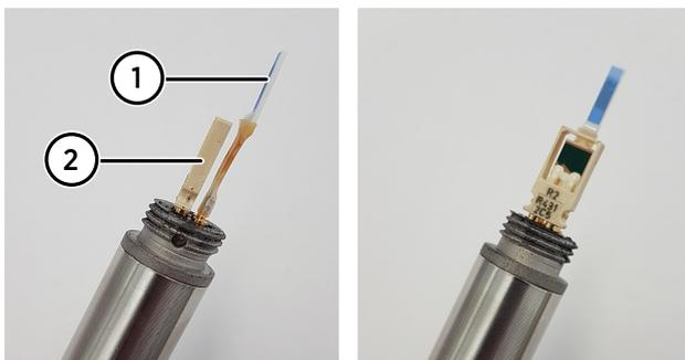
Figure 29 HMP3 probe head with filter removed
