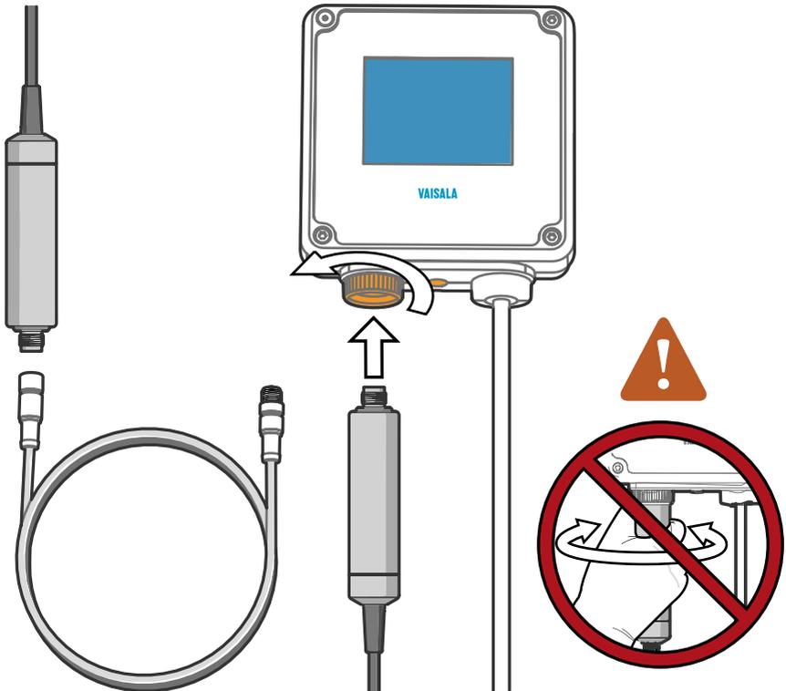
Figure 27 Attaching the probe to Indigo200 series transmitter
