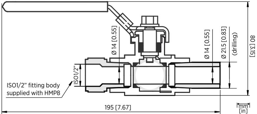
Figure 51 Optional ball valve installation kit dimensions
