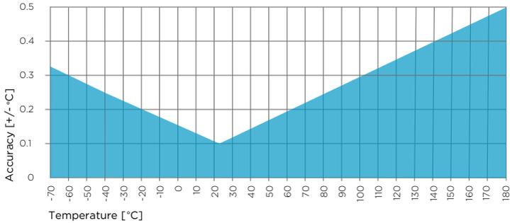
Figure 46 HMP7 temperature measurement accuracy over full range
