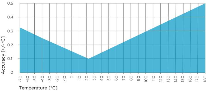
Figure 49 HMP8 temperature measurement accuracy over full range
