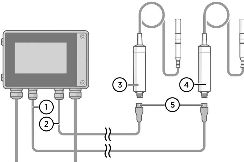
Figure 21 Connecting probes to Indigo500 transmitter
