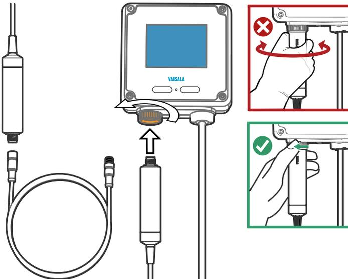
Figure 19 Connecting probe to Indigo200 series transmitter
