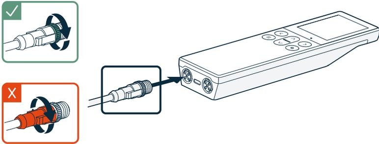
3. Connect the probe to the M12-5F end of the probe connection cable.
