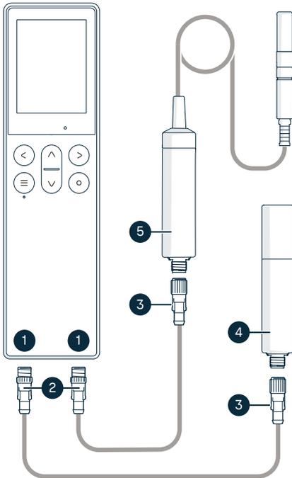
Figure 23 Example of connecting probes to Indigo80
