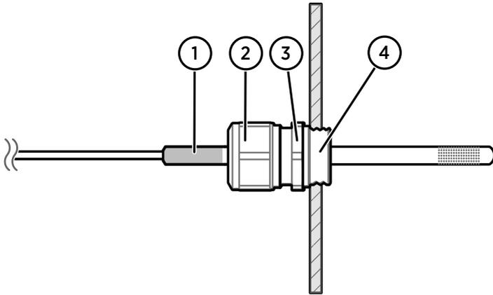
Figure 16 Installing HMP9 probe head through a cable gland
