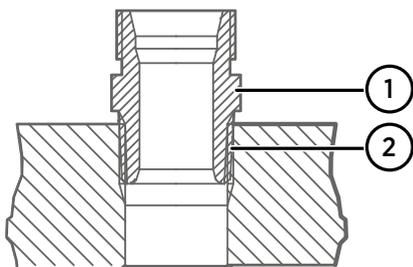
Figure 14 Sealing of fitting body into process
