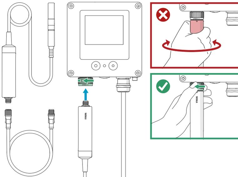
Figure 20 Connecting probe to Indigo300 transmitter
