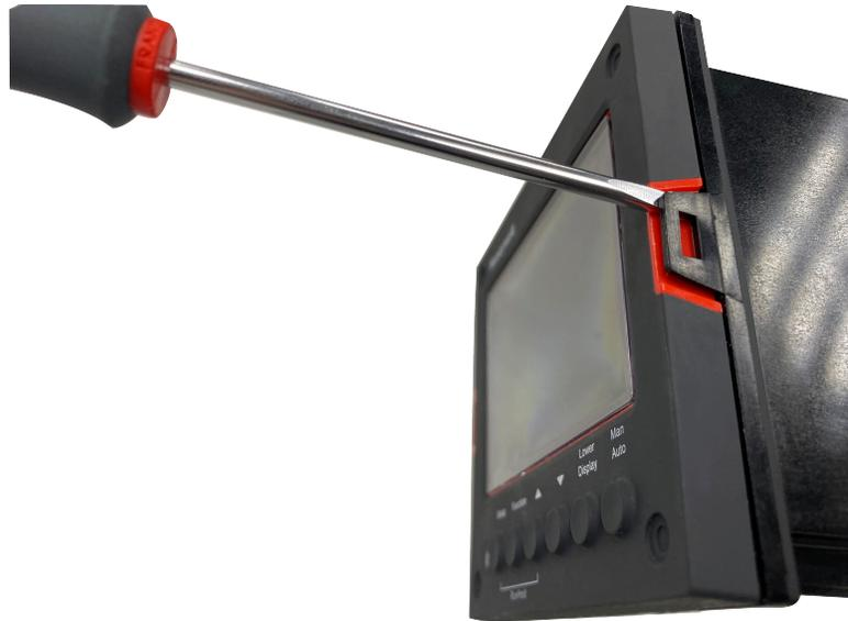
Using a thin screwdriver, gently twist the screwdriver to pry the side tabs from the front face. Pry just enough to release it, otherwise you'll bend or break the tab . If you break or bend the tab and can't reattach the front snugly, you'll need to reattach the front using the 4 NEMA4 screws provided. See "Mounting" on page 46 for more information.
