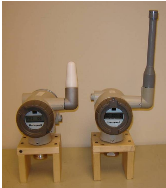
Figure 6-1 Comparison of instruments with -2 dBi Integral Antenna (left) and 4 dBi Integral Antenna
