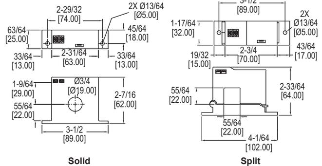
The **Series CCT40/50 Current Transformers** are a low cost alternative for measuring power and monitoring the operation of fans, pumps, or other equipment. For use on existing installations, split core models can be installed without disconnecting cables. Each model offers three jumper selectable ranges and a choice of three different outputs.
