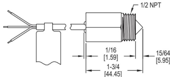
The **Series OLS Optitrol® Optical Level Switches** are low cost, rugged optical level switches that indicate the presence or absence of liquid via infrared light that is reflected back through the prism lens. This series offers three optional materials, 316 SS, polysulfone and PFA.
