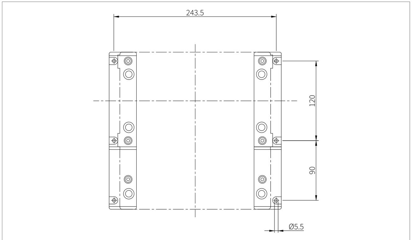
Picture 7: Drilling aid for wall mounting KATflow 150
