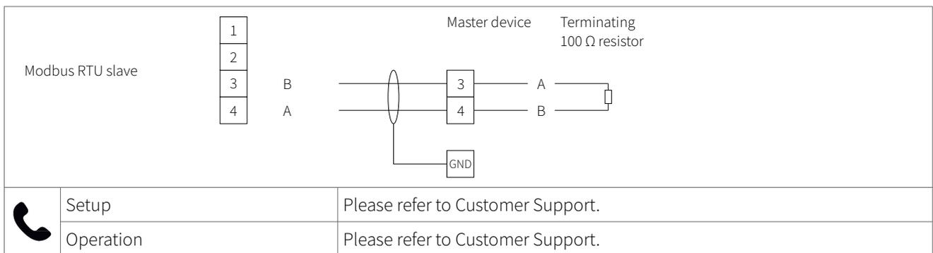
Table 18: Wiring Modbus RTU
