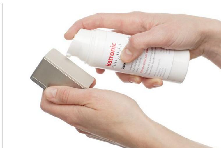
Picture 7: Application of acoustic coupling gel
