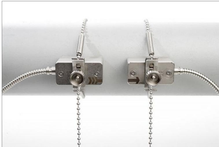
Picture 8: Correct positioning of the sensors
