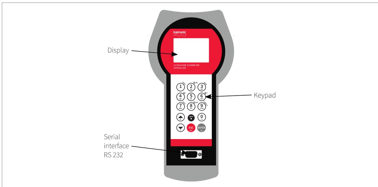
Picture 12: Keypad and display KATflow 200
